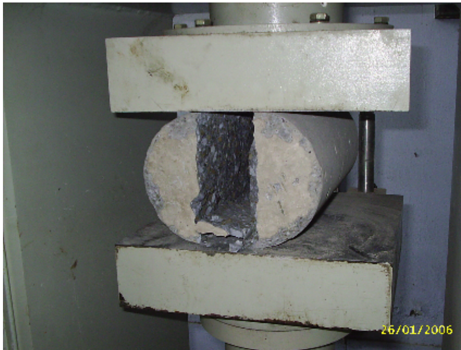
Plate 3.6. Failure patterns in split tensile test
