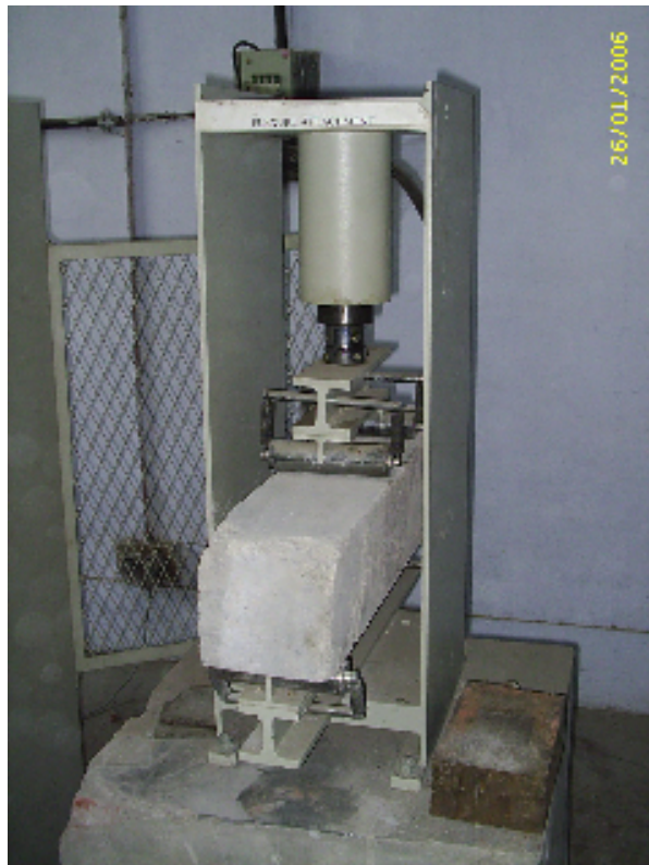
Plate 3.4. Typical arrangement for flexure test
