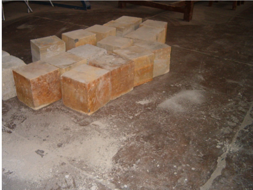
Plate 5.1. Brownish belt that appeared on the specimens exposed to hydrochloric acid attack
