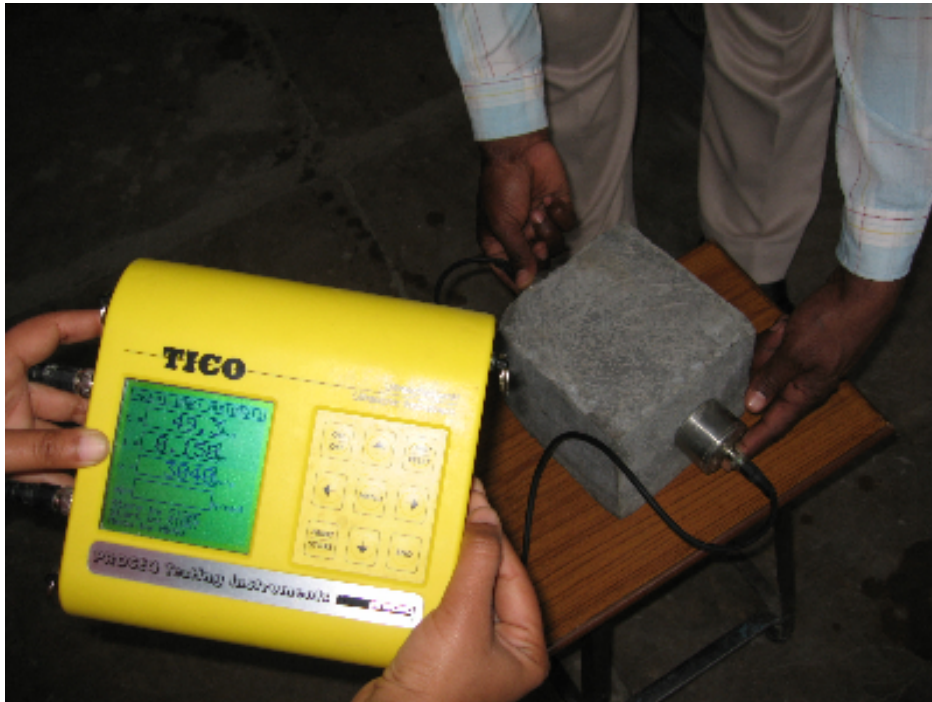
Plate 3.8. Ultrasonic pulse velocity test in progress
