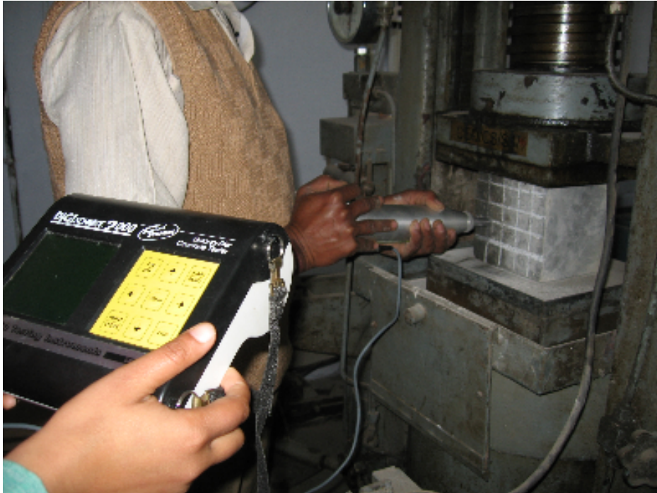
Plate 3.7. Rebound hammer test in progress
