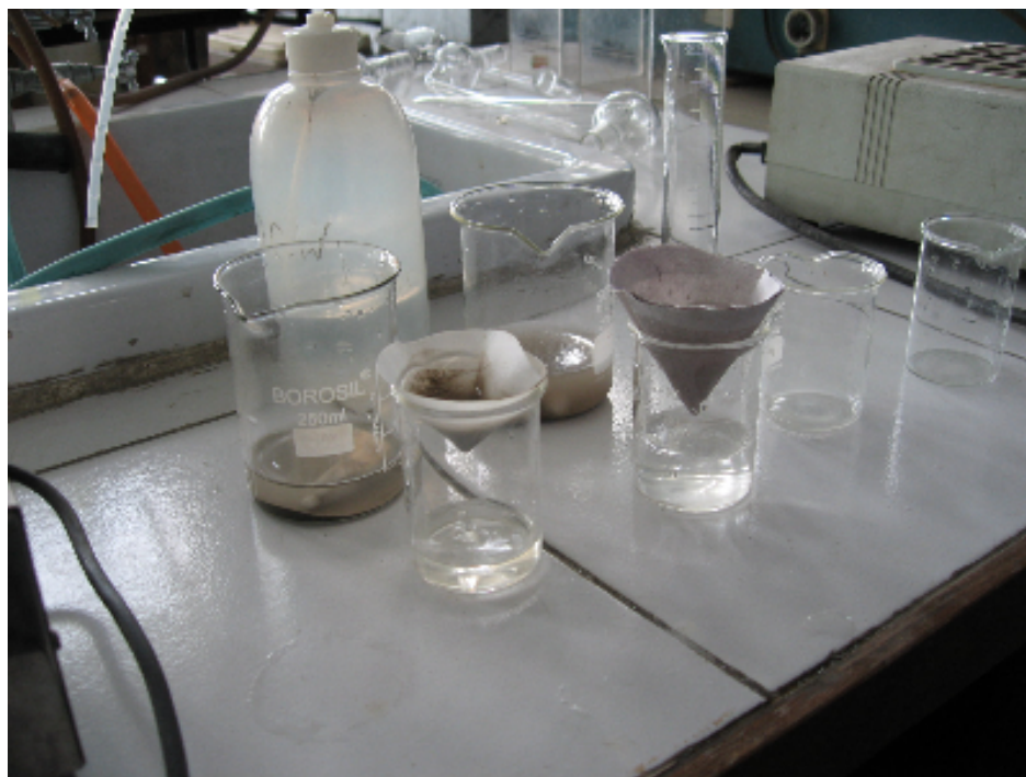
Plate 3.21. Filtering of samples after stirring
