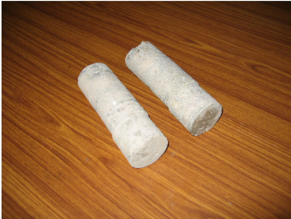
Plate 3.16. Typical cores used for chloride analysis at various depths
