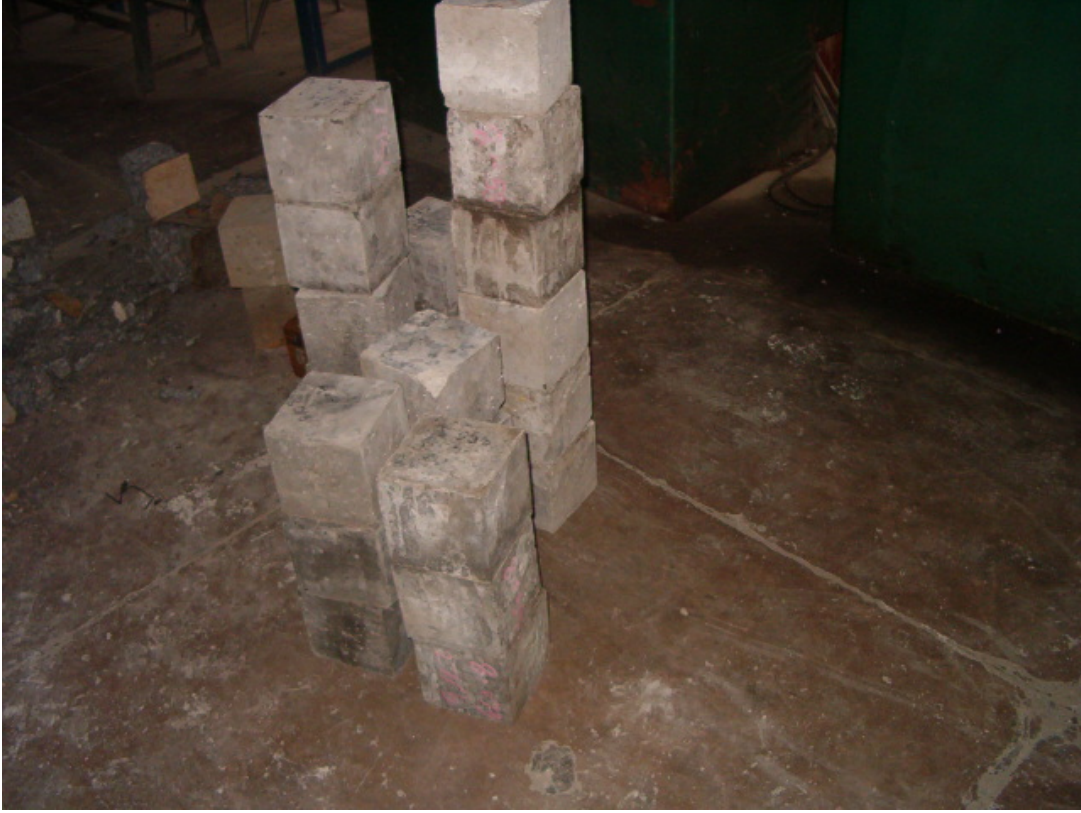
Plate 5.3. White deposits on the surface of specimens exposed to magnesium sulfate solution
