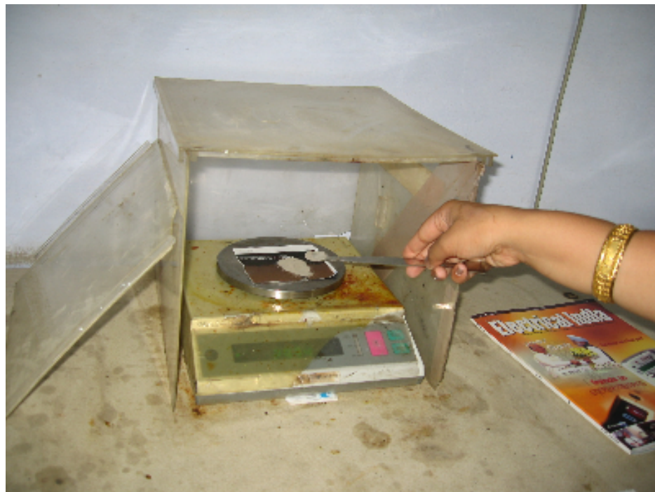
Plate 3.19. Collection of 3 gram sample for chloride analysis
