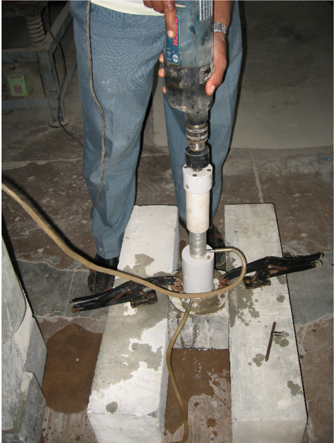
Plate 3.13. Positioning of diamond core cutter for taking cores
