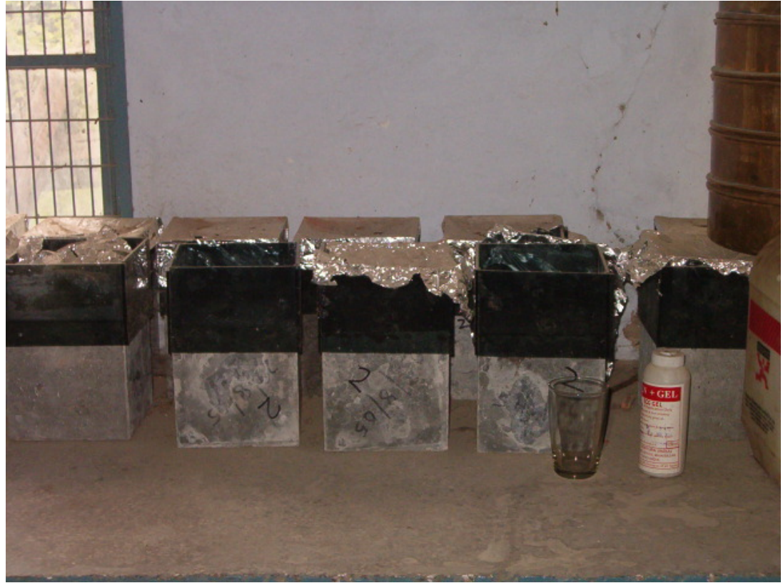
Plate 3.12. Dykes prepared at the top of the specimens for ponding chloride solution
