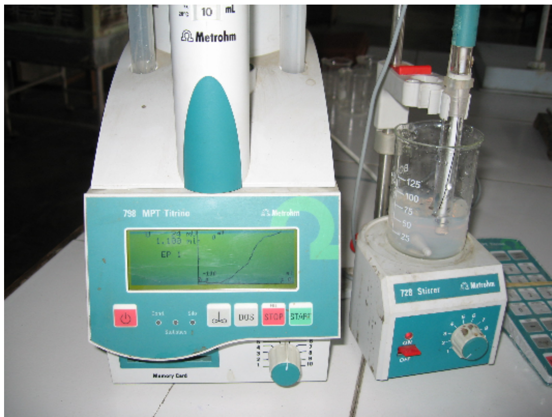
Plate 3.22. Typical potential vs titration volume plot for obtaining end point
