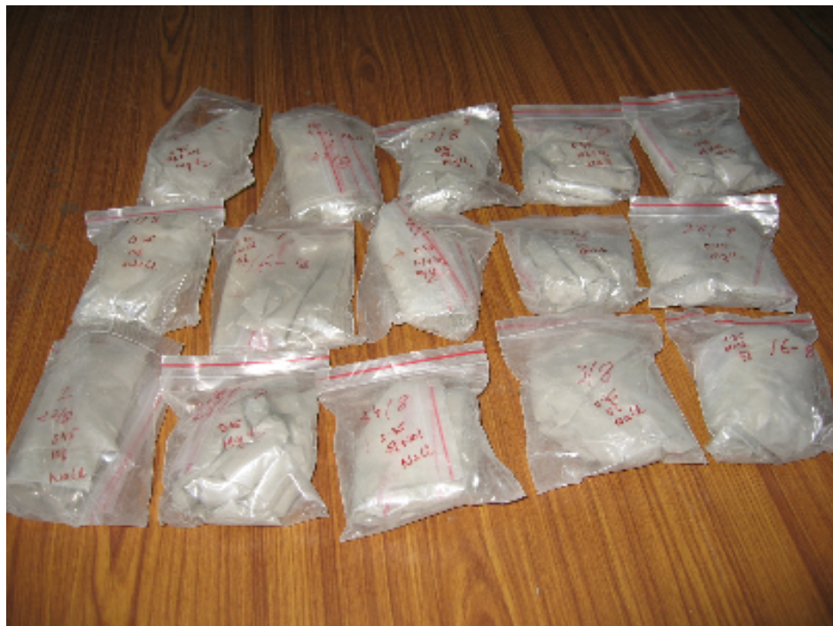
Plate 3.17. Powder concrete samples collected from various depths of cores for chemical analysis
