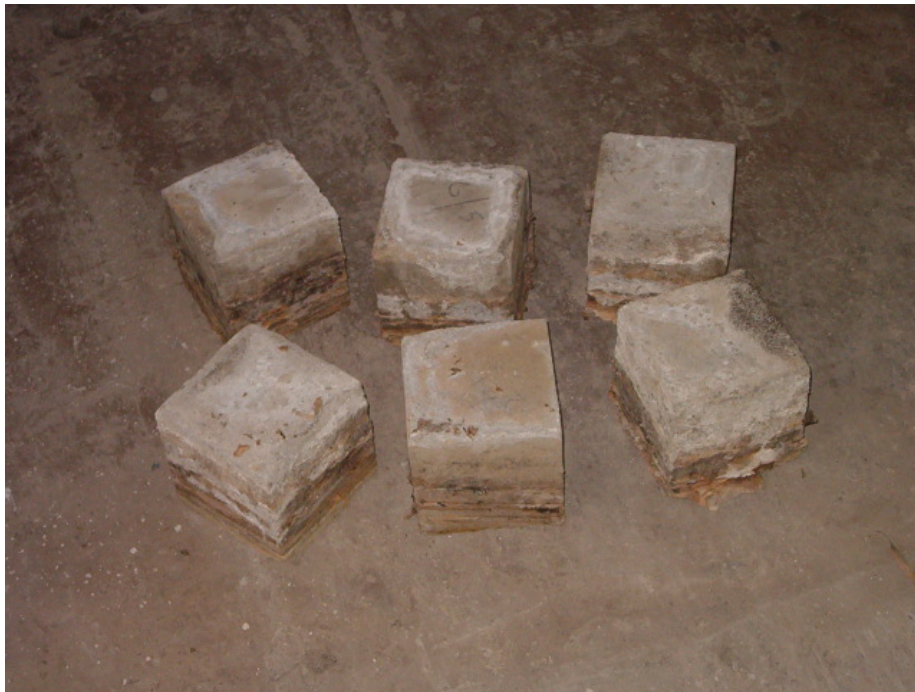
Plate 5.1. Brownish belt that appeared on the specimens exposed to hydrochloric acid attack
