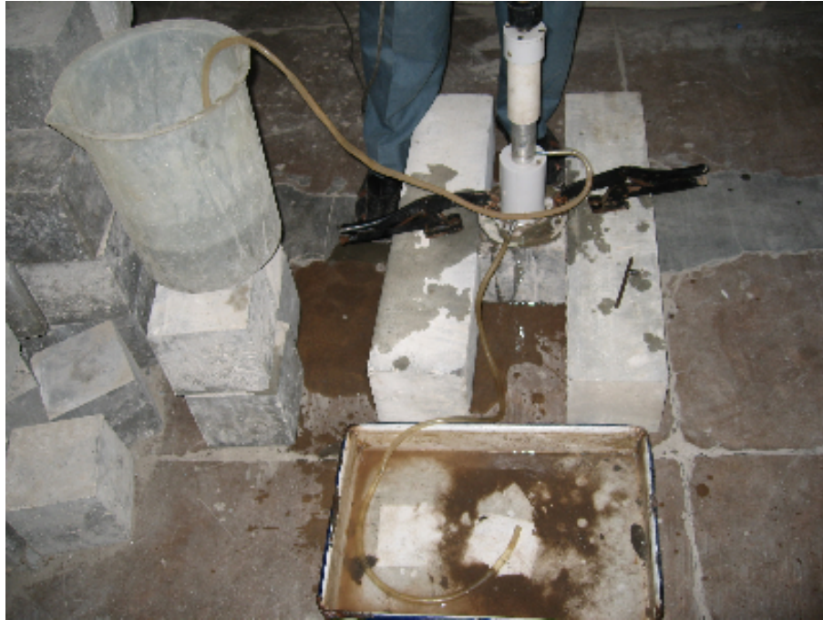
Plate 3.14. Core cutting in progress
