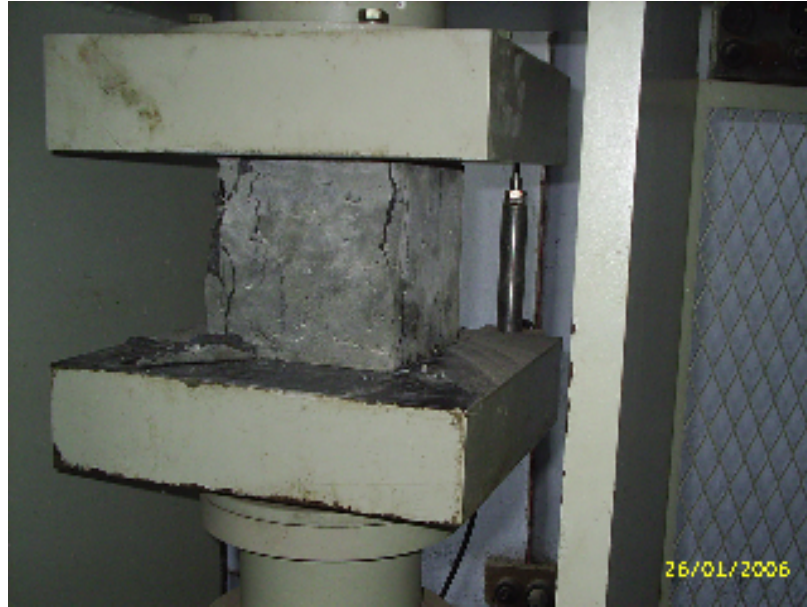
Plate 3.3. Compression test in progress
