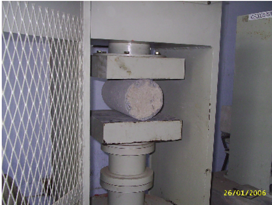
Plate 3.5. Split tensile test on cylindrical specimens in progress
