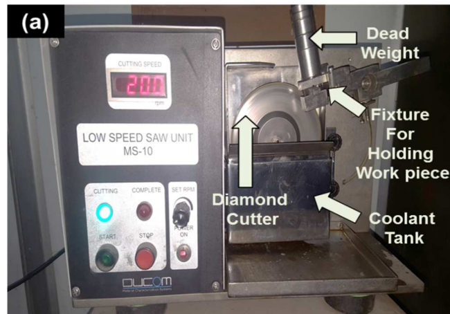
Figure 5.7: Low speed saw unit ( Photo Courtesy: Surface Engineering and Tribology Research Lab, Mechanical Engineering Department, TIET, Patiala )
