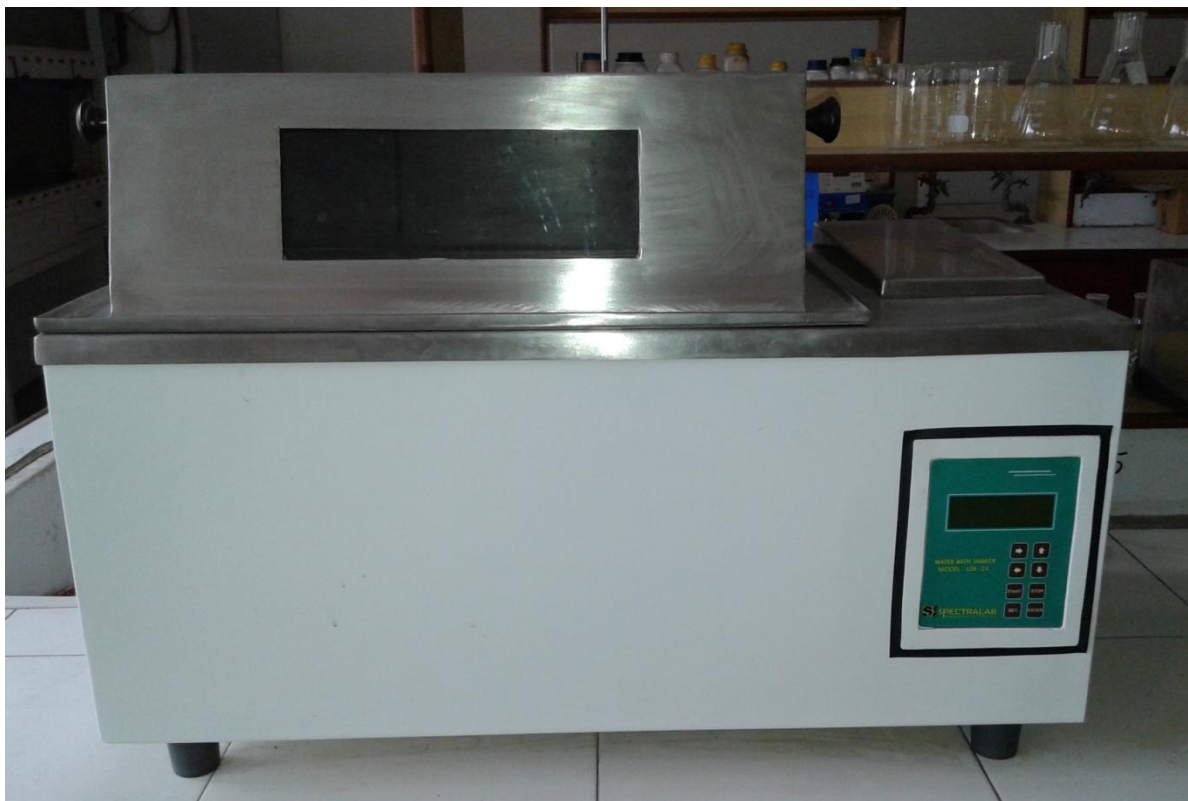
Fig.3.1. Temperature controlled water shaker bath (LSB-24) of Spectralab, India.
