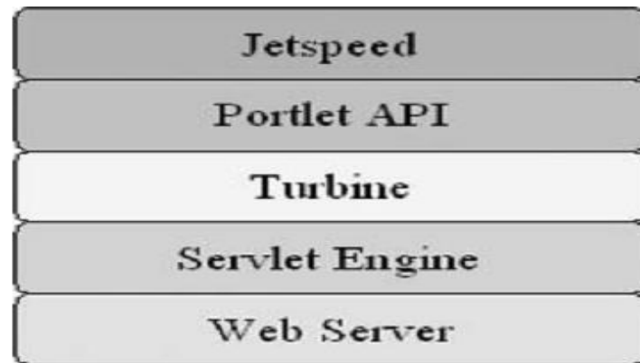
Figure 2.7: The Architecture of Jetspeed [1]
