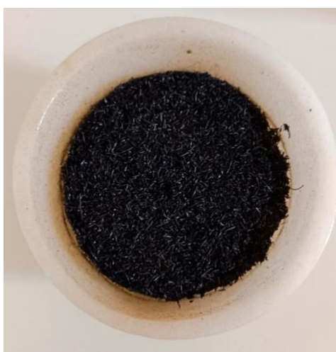
Figure 2 : BC Produced after Pyrolysis at 400°C
