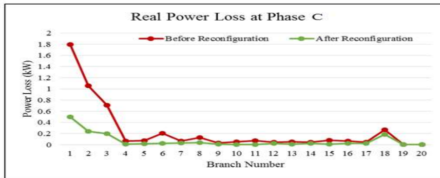
(c) Real power loss at phase C
