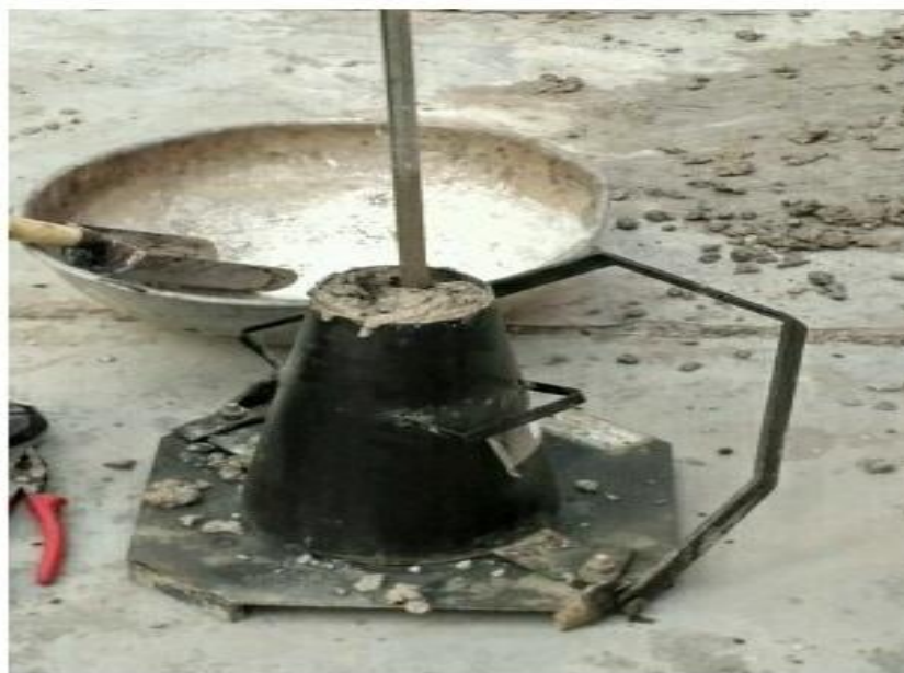
Fig.3.7: Experimental set up for measuring workability by using slump cone
