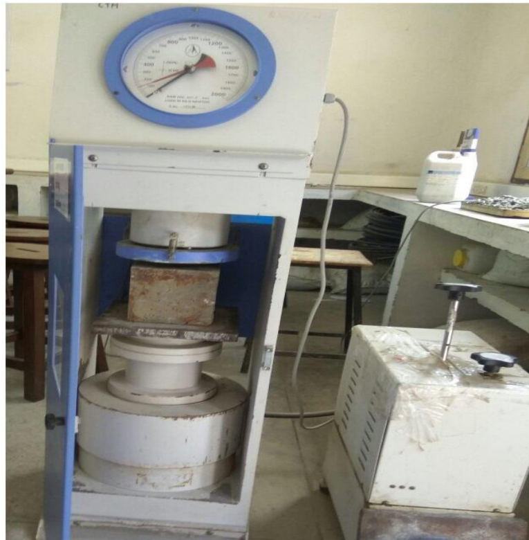
Fig.3.10: Experimental set up for measuring compressive strength
