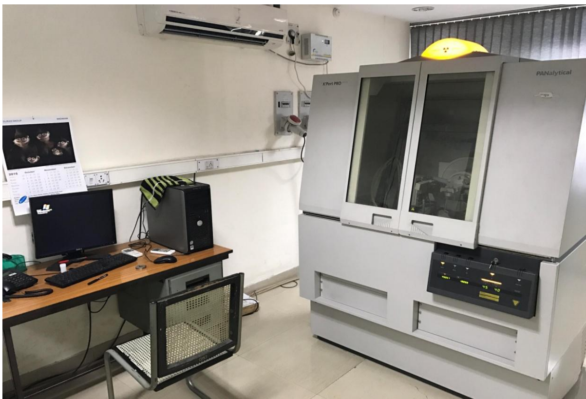
Fig.3.17: Experimental setup for XRD analysis
