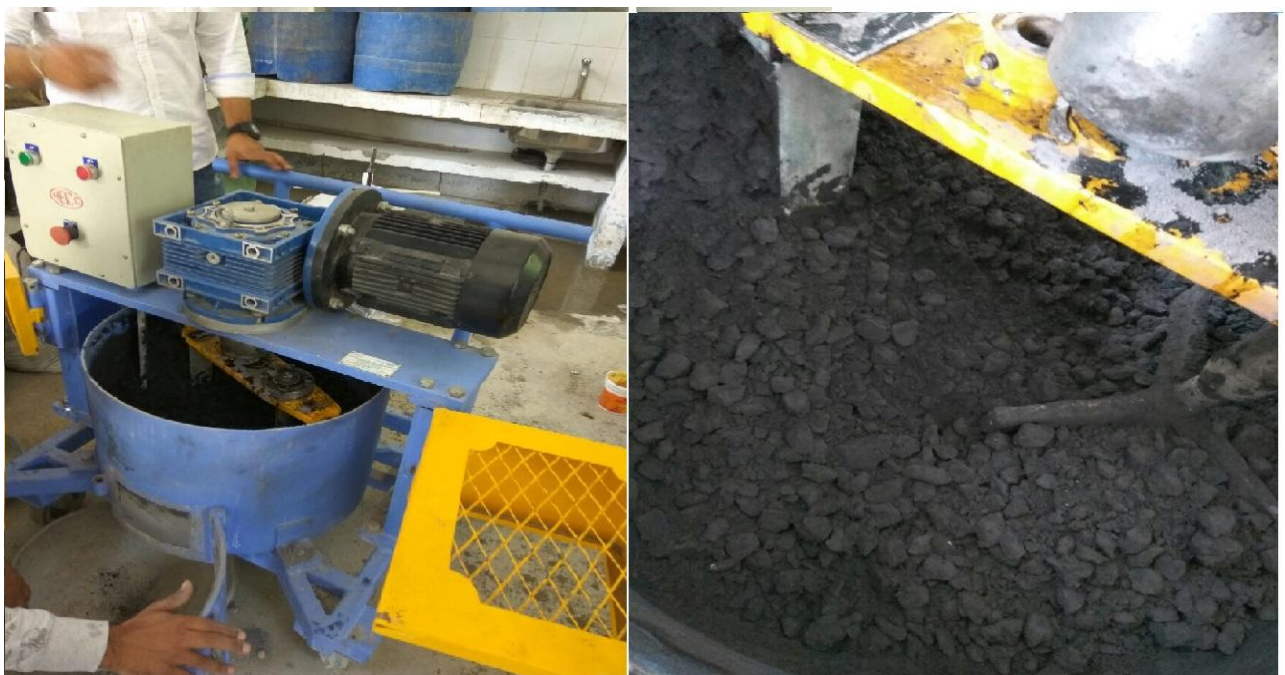
Fig.3.6: Making of concrete in a pan mixture
