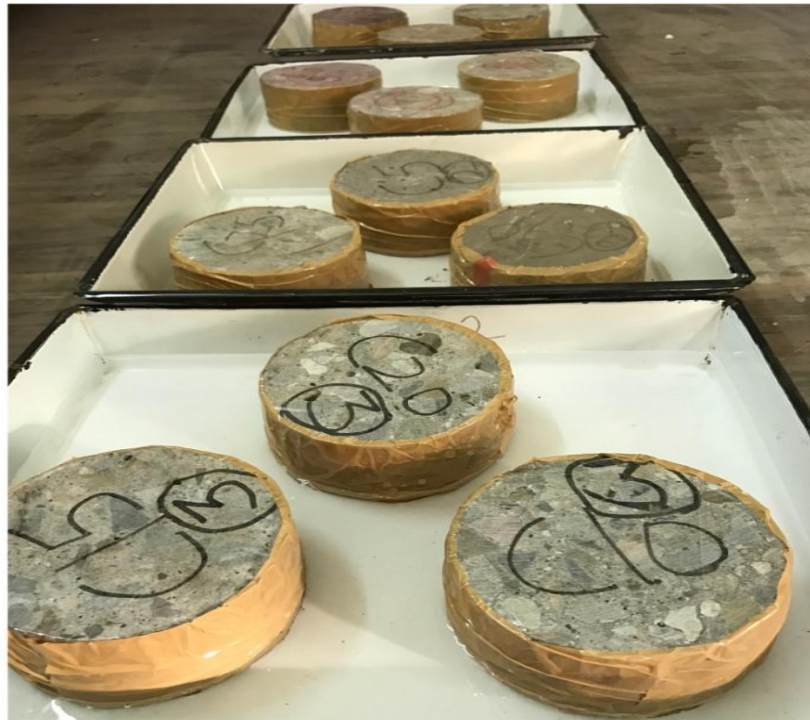
Fig.3.12: Experimental set up for measuring sorptivity of concrete
