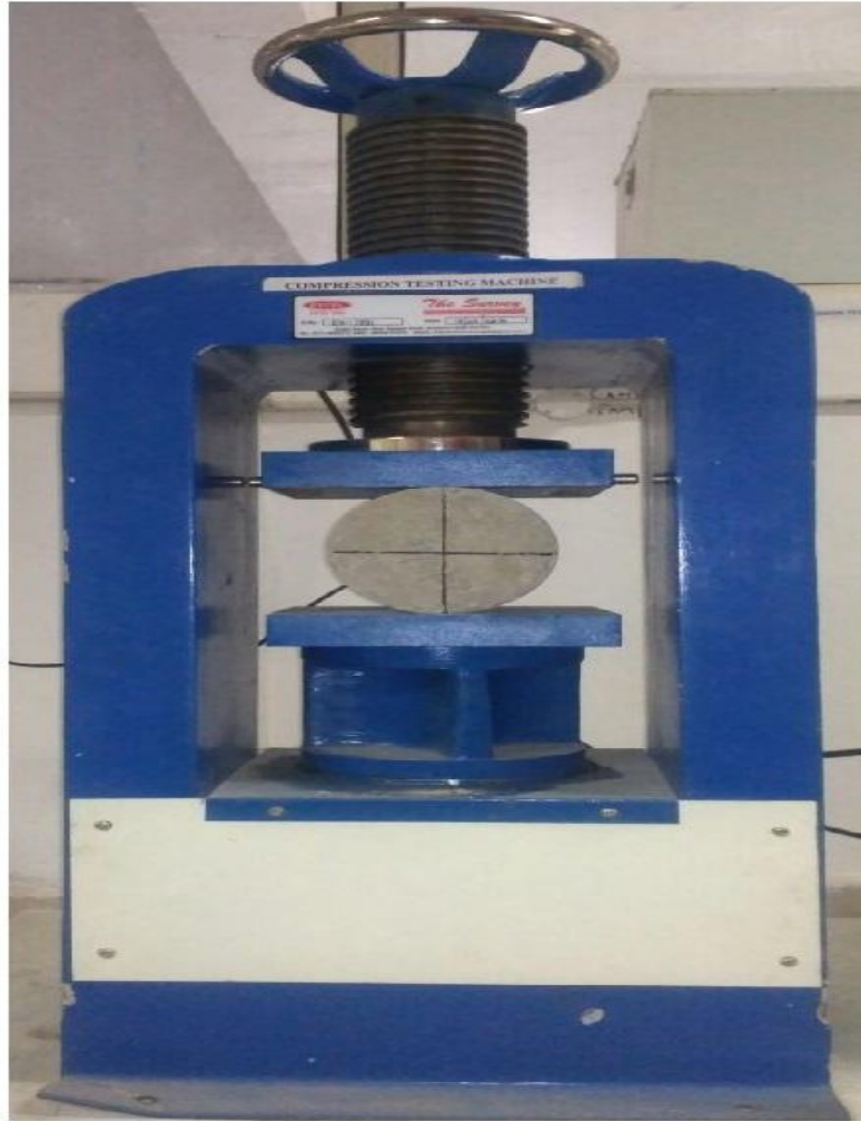
Fig.3.11: Experimental set up for measuring split tensile strength
