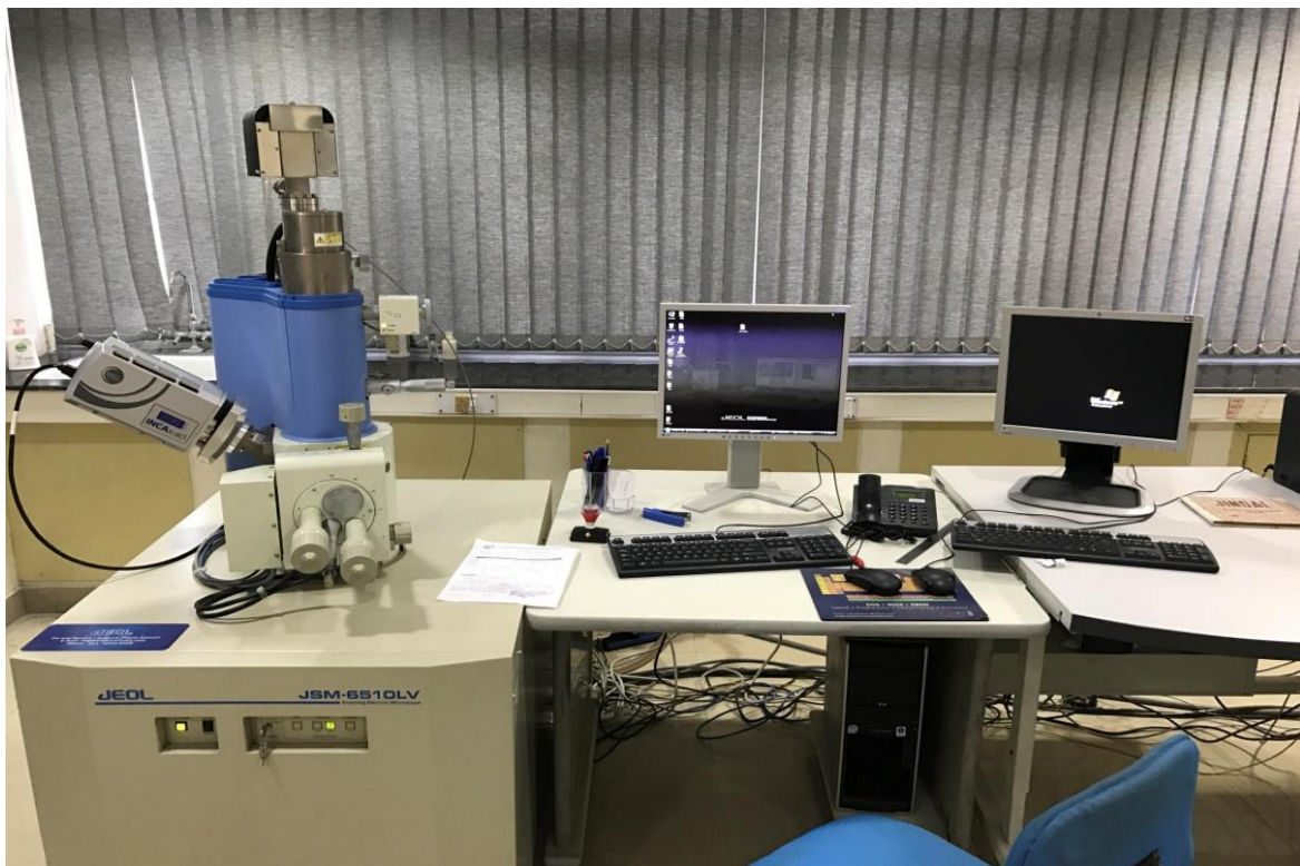
Fig.3.15: Experimental setup for Scanning Electron Micrograph
