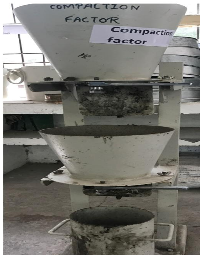
Fig.3.9: Experimental set up for measuring workability by using compaction factor
