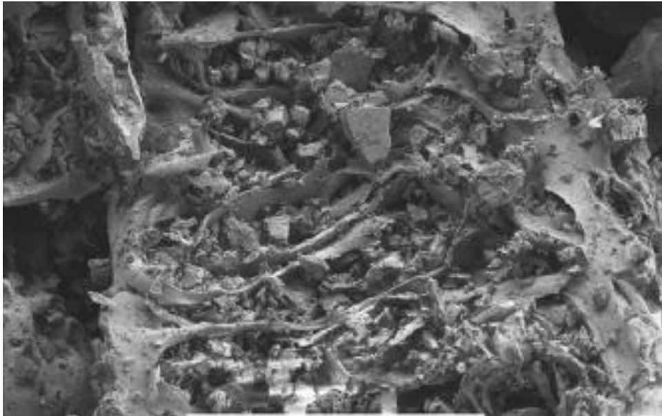
Fig.1.8: Scanning electron microscope micrographs of rice husk ash (Kusbiantoro et al., 2012)
