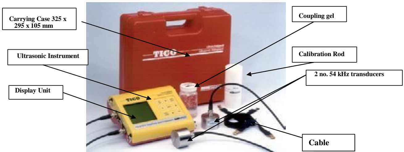
Fig 4.18 Components of TICO Ultrasonic Instrument
