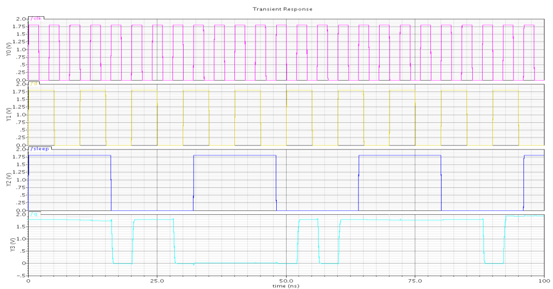
Fig. 3.3.1(b) Simulation of low power TSPC rising edge flip-flop.
