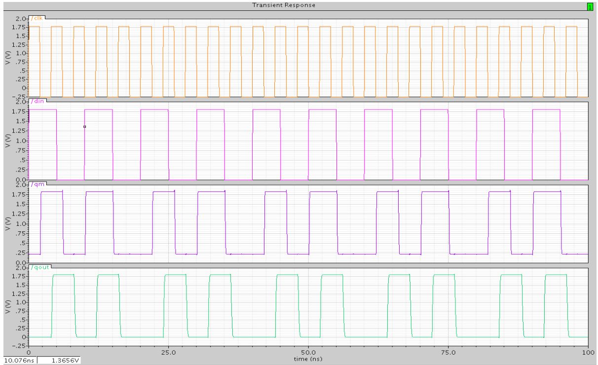
Fig. 3.2(b) Simulation of rising edge triggered master slave flip-flop.
