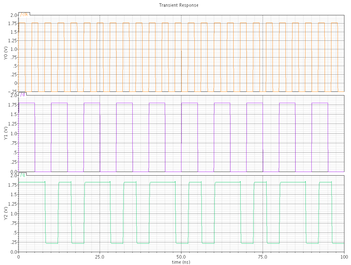
Fig. 3.3 (b) Simulation of TSPC rising edge flip-flop.
