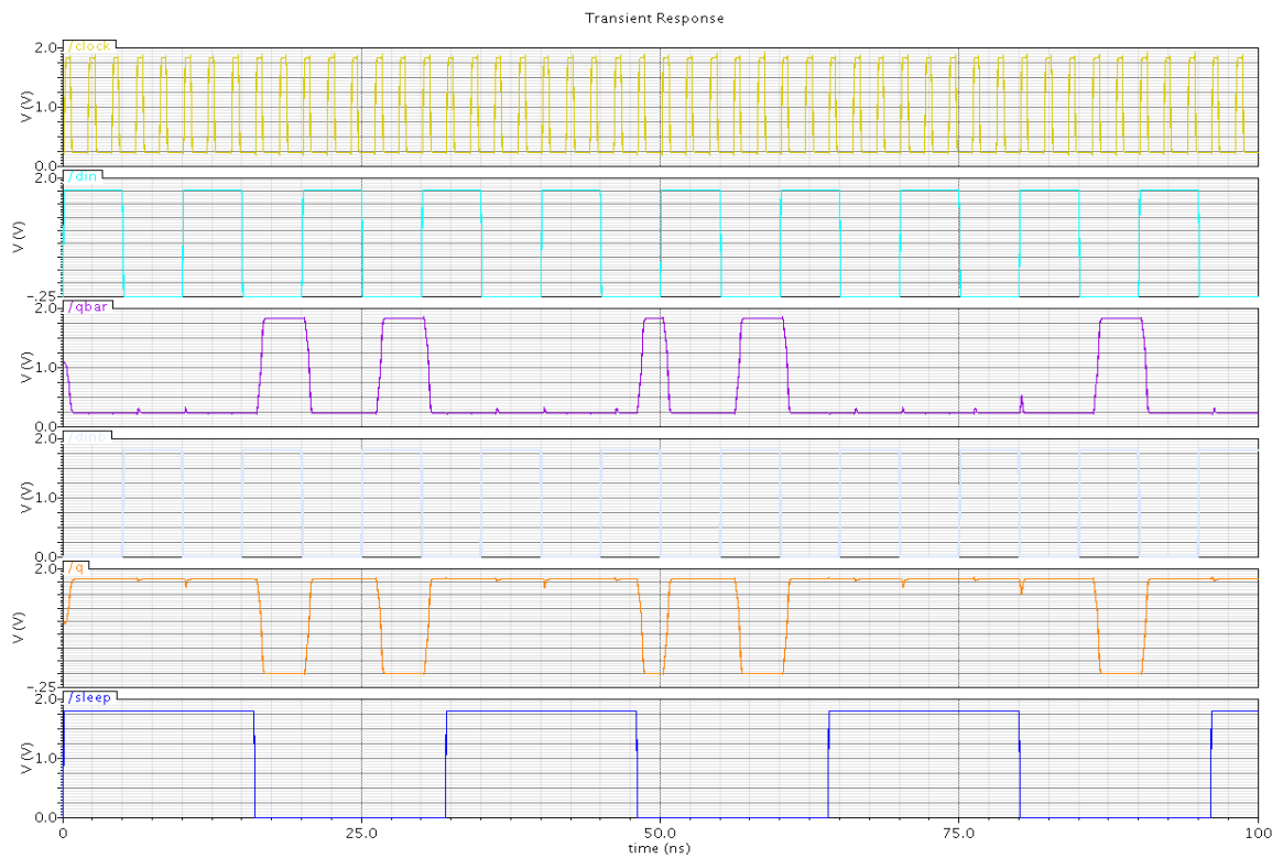
Fig. 3.4(c) Simulation of pulse static dual edge triggered flip-flop.
