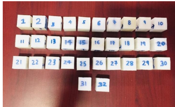
Figure 3.5: Nylon parts fabricated by 3d printer (30×30×30mm)
