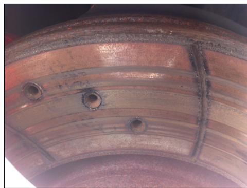
Figure 1.4: Scarring in disc brake [40]
