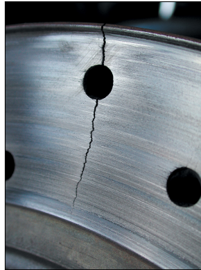
Figure 1.5: Cracking in disc brake [41]
