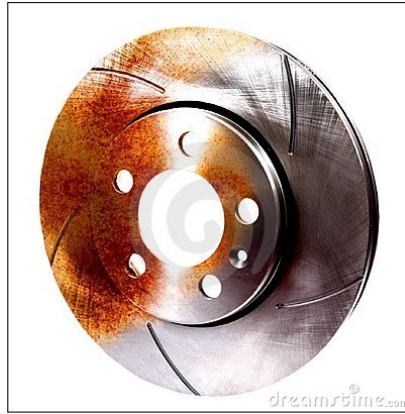
Figure 1.6: Rusting in disc brake [42]
