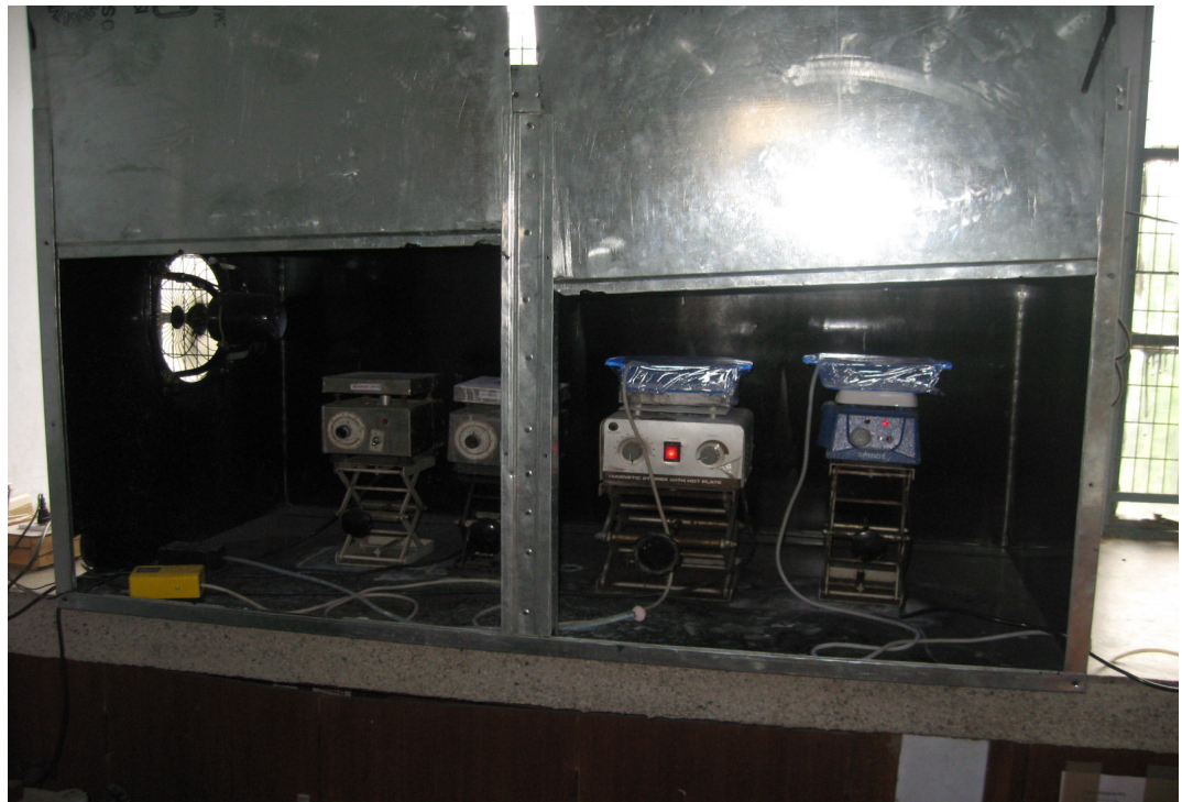
Fig-3.2.1 b Photoreactor at lab level during photocatalytic treatment
