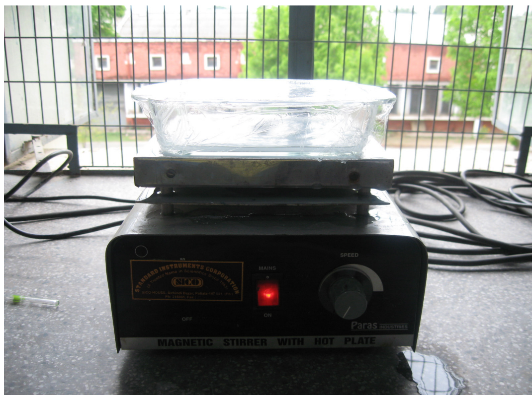
Fig-3.2.3 Glass bowl reactor with magnetic stirrer at lab scale
