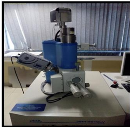
Figure 3.6 SEM equipment equipped with EDS (Photo courtesy: SAI Labs, TIET, and Patiala)
