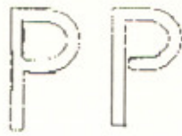
Figure 1.1 : Example of two characters that look quite similar but they are topologically different
