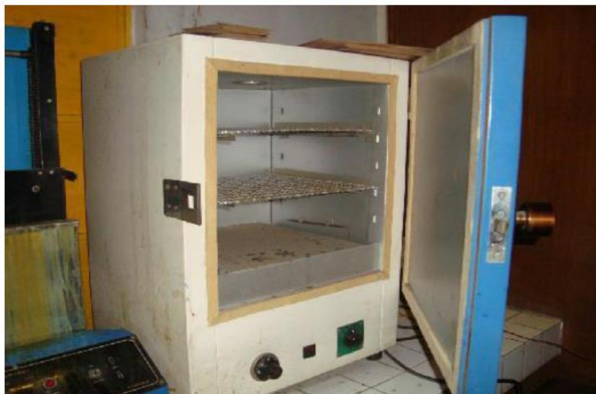
Figure 4.3 Oven unit used for drying process
