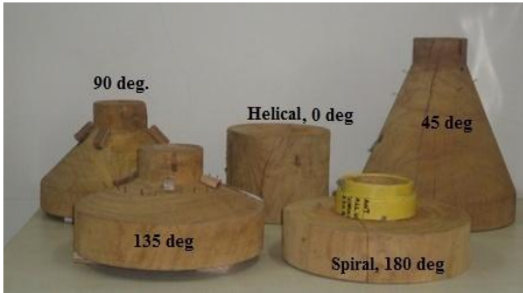
Fig. 3.1 Conical coil formers for coil fabrication
