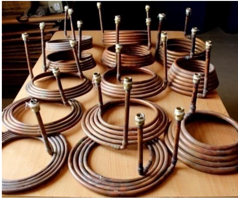
Fig. 3.2 Conical coils fabricated for analysis
