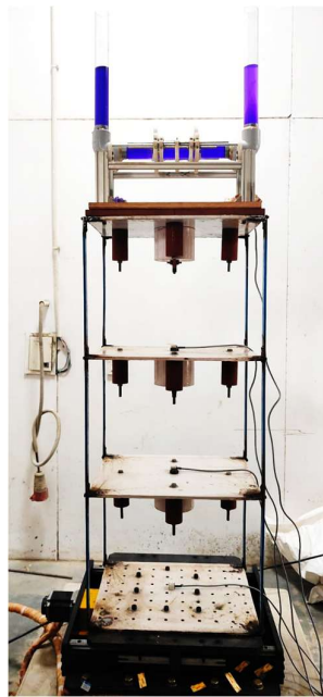
Figure 3.3: Representation of the building with the CTLCD with load provision on each story, placed shake table experimental model.
