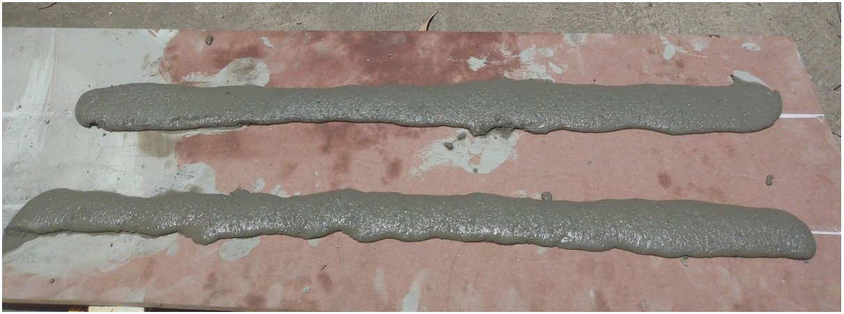
Fig 4.3 Extruded Filaments from 3-D Printer
