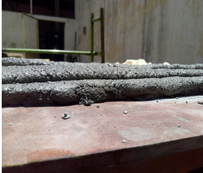
Fig 4.5: Un-deformed Layers (Buildable)
