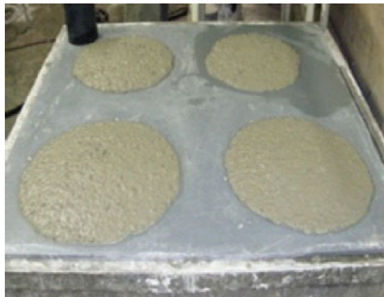
Fig 2.2: Spread of mortar at four spread of USS test
