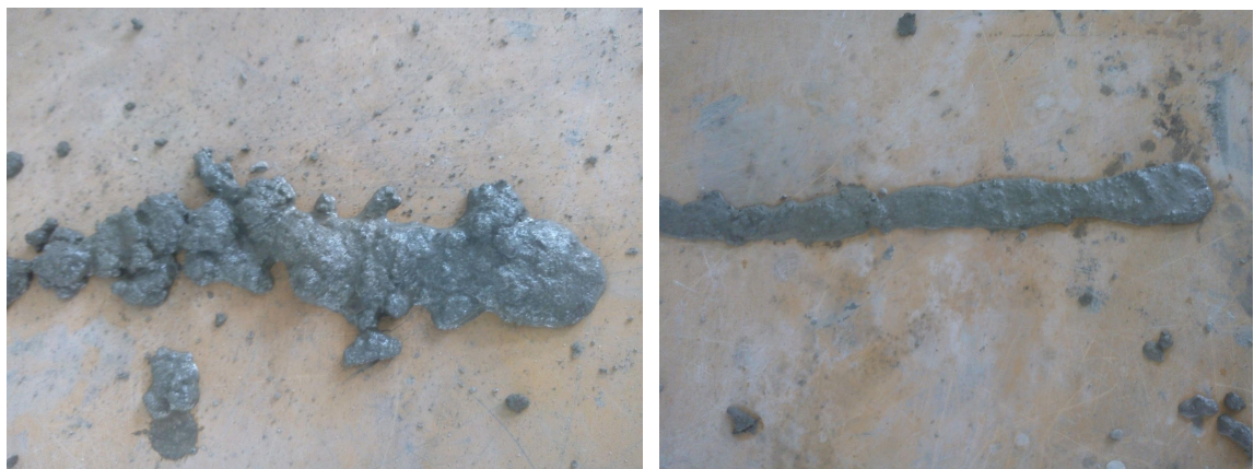
Fig 4.2: (a) Un-Extruded Mix (b) Extruded Mix
