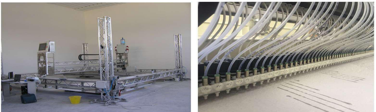
Fig:1.3 D Shape 3-D printer (left) printing head (right).
