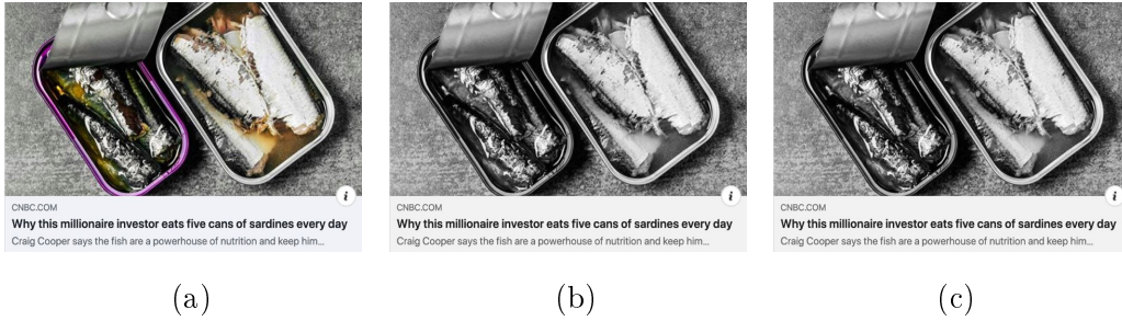
Figure (4.4) Pre-processing on (a) Original image, (b) Grayscale image and (c) Denoised image
