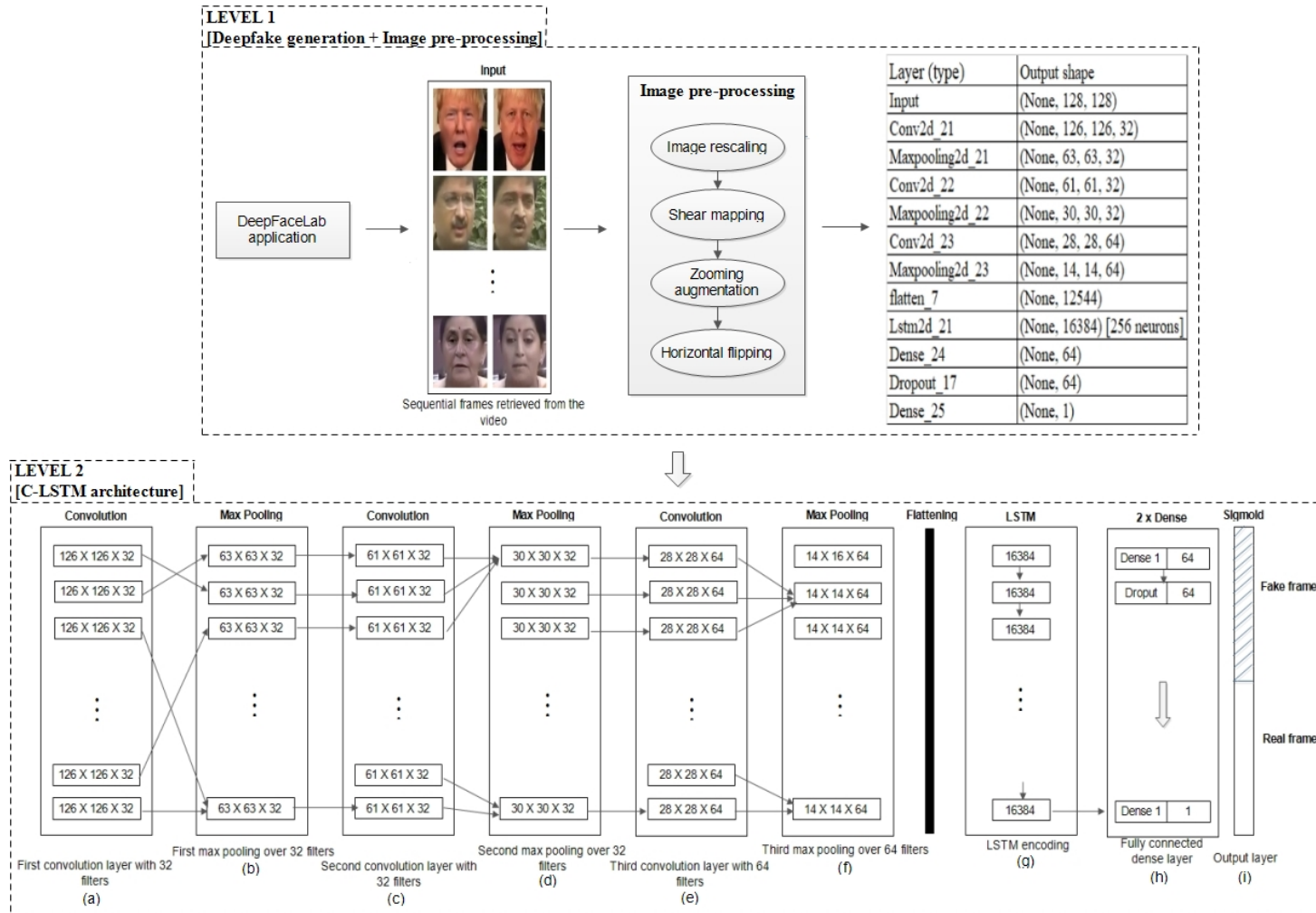
Figure (5.9) Two-level structure of the proposed deep temporal-based C-LSTM model for automatic detection of deepfake face-swapped video clips of politicians
