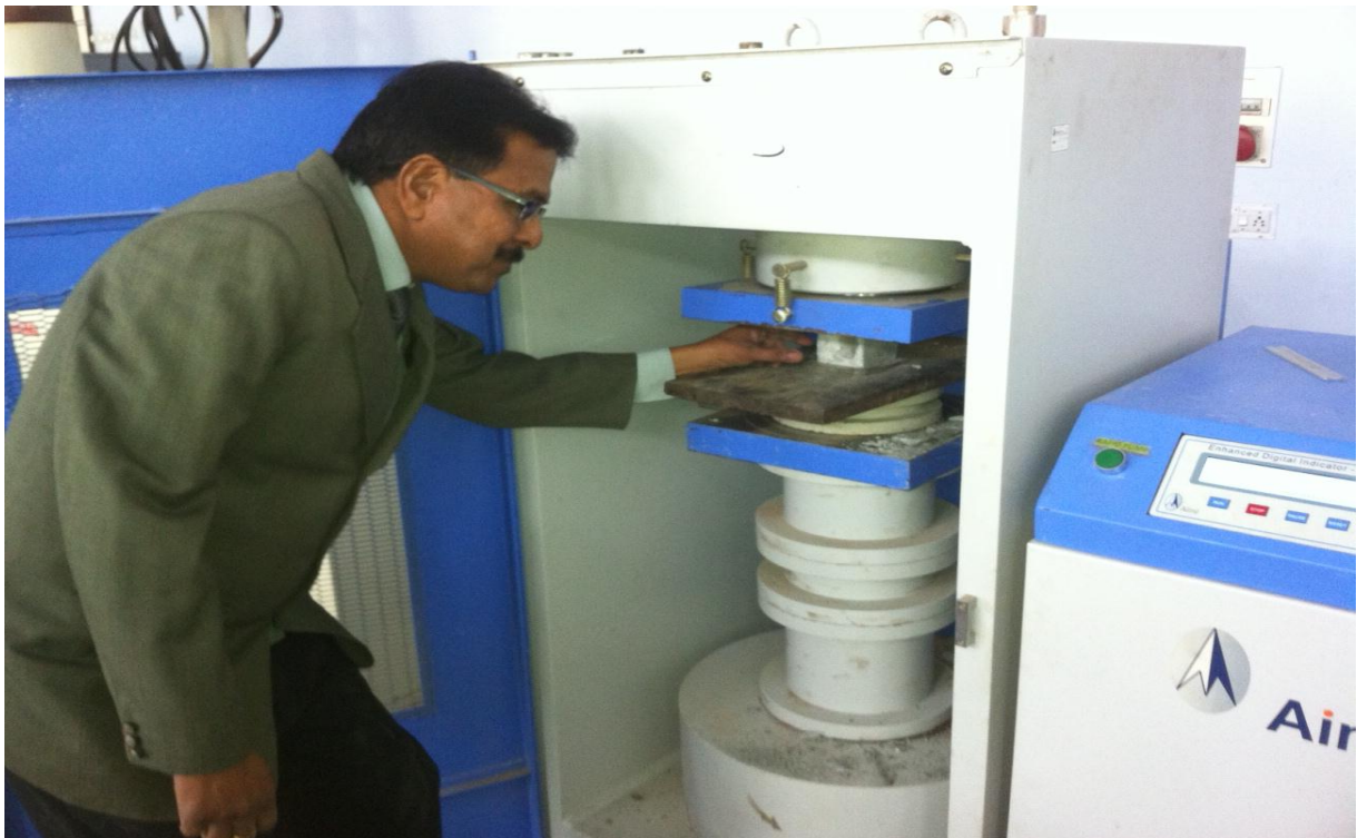
Fig. 5.3 Cement Mortar Cubes being tested by Compression Testing
