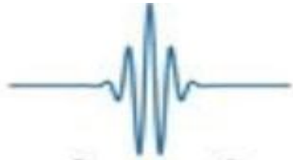
Fig. 4.2 The wavelet for small scale factor with high frequency
