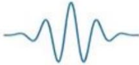
Fig. 4.1 The wavelet for large scale factor with low frequency
