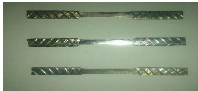
Figure 3.4: Specimens for Tensile test
