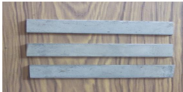
Figure 3.1: Bending test Specimens
