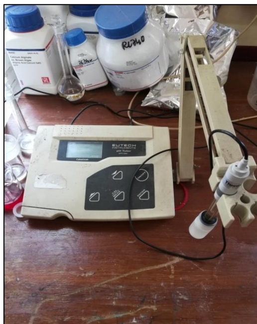
Fig. 5.2 – pH get adjusted by Eutech pH meter
