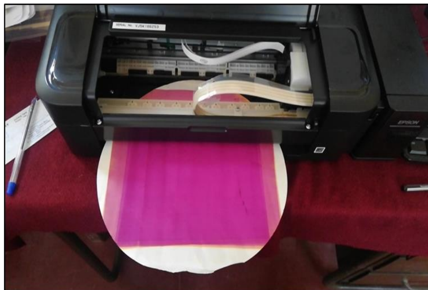
Fig. 5.3 - Dye get printed on whatman filter paper by using Epson L360
