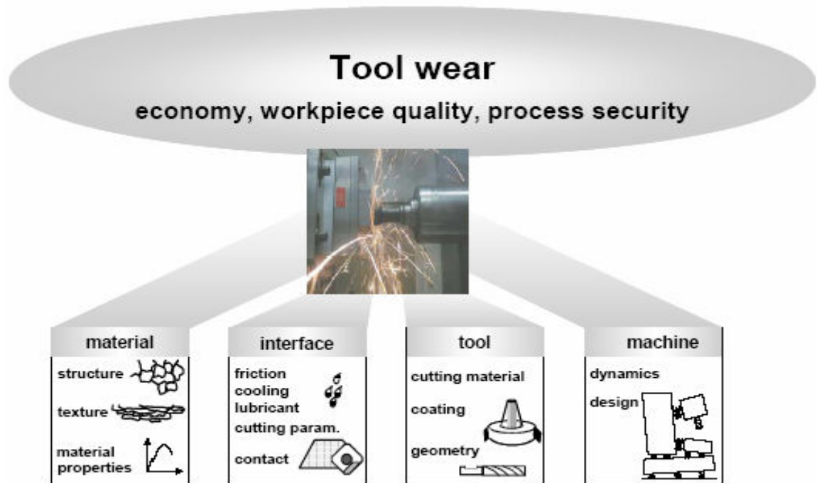
Figure 1.4: Influencing elements of tool wear
