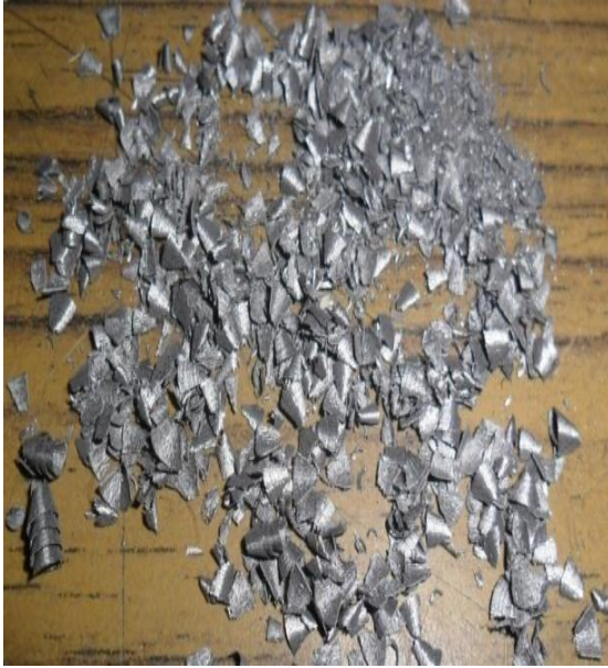
(a) Natural broken Chips produced at Exp. No 13
