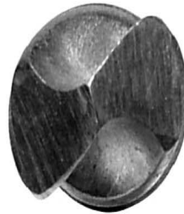
(b) Exploded view of cutting edge for twist drill
