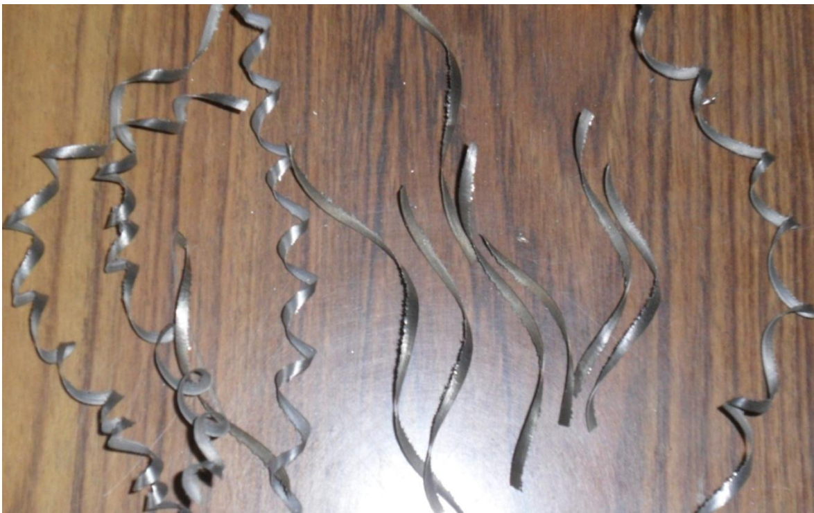
Figure 7.7 Long ribbon types of chips produced during machining H 11-work piece at 244 rpm
