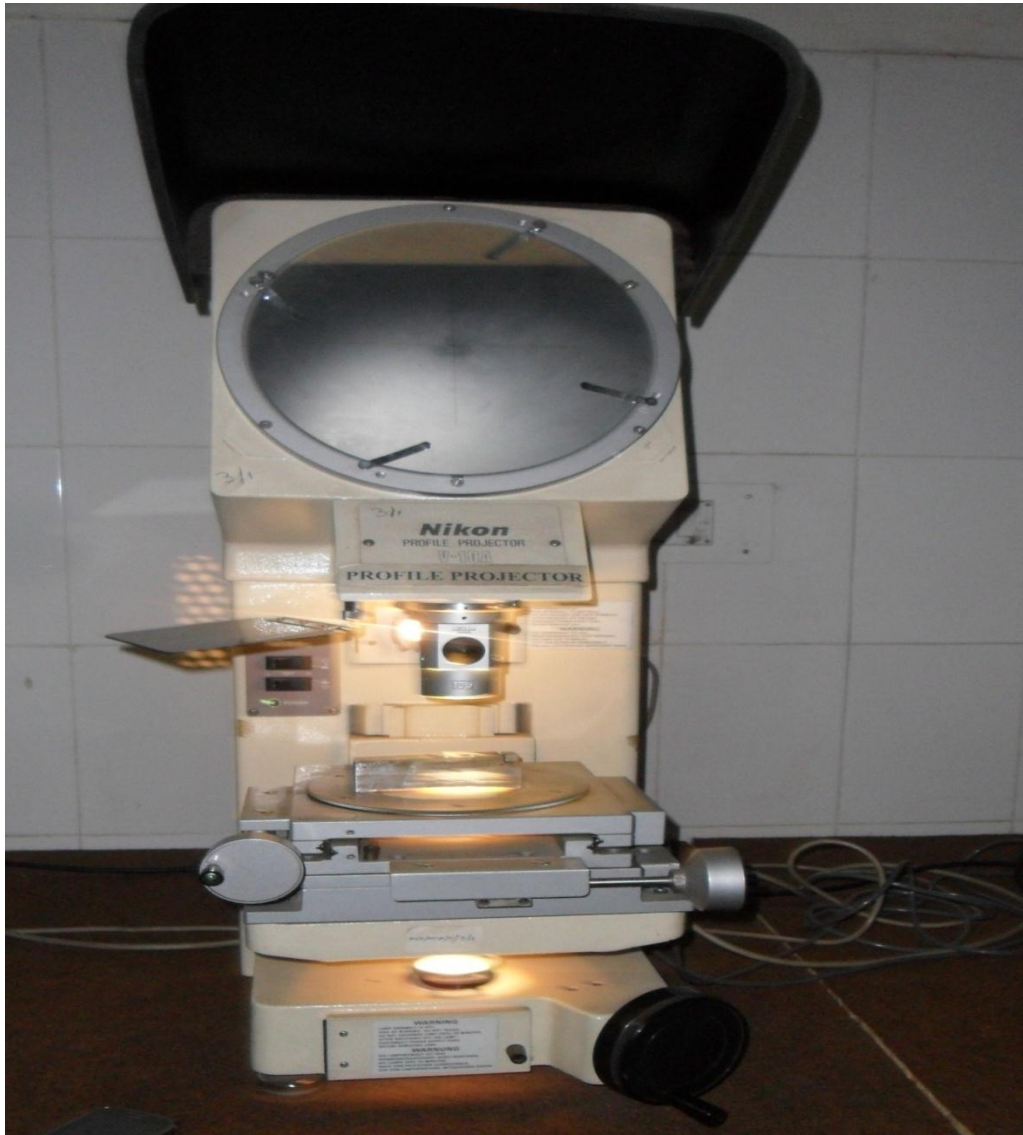
Figure: 3.5 Device for measurement of hole diameter accuracy (Source: Metrology lab, TU, Patiala)
