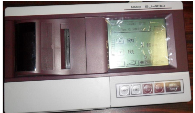
Figure: 3.4 Experimental devices for measurement of surface roughness (Source: Mechanical Engineering Department, TU, Patiala)
