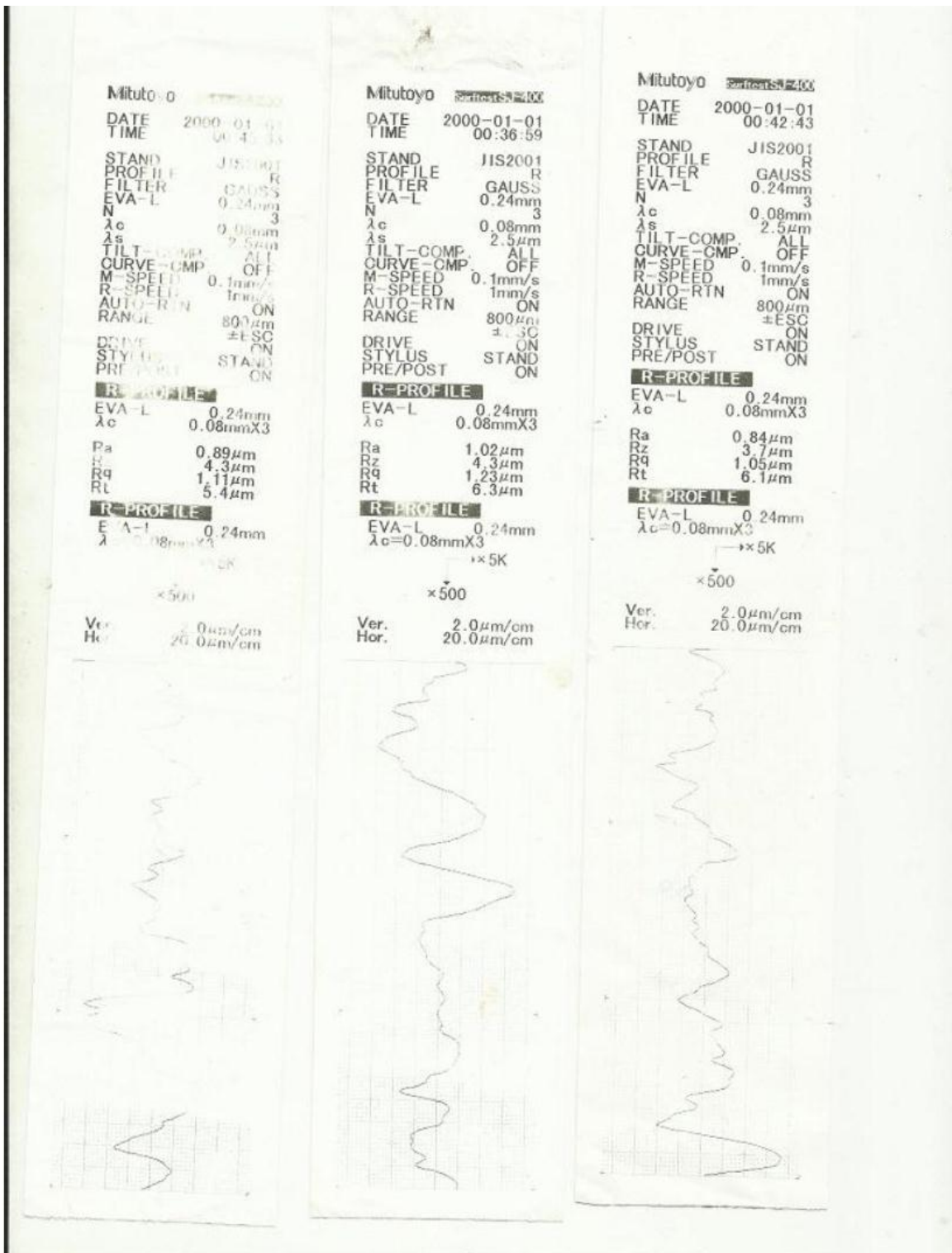
Figure 5.1 Profile of surface roughness for experiment no 5, 10 and 16 respectively.
