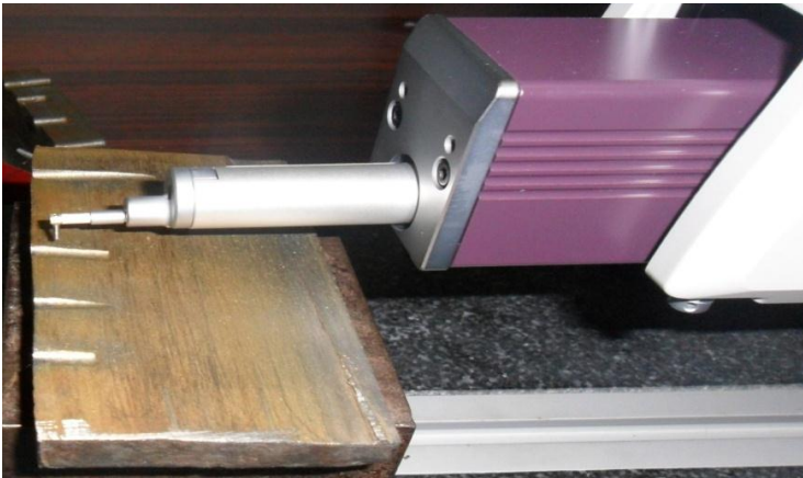
Figure: 3.4 Experimental devices for measurement of surface roughness (Source: Mechanical Engineering Department, TU, Patiala)
