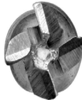
(d) Exploded view of cutting edge for 4-flute cutter
