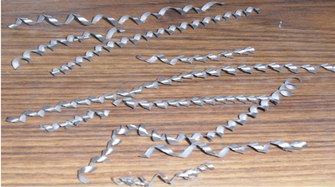
Figure: 7.6 conical helical chips are producing during machining EN 31-work piece at 244 rpm, 0.15 mm feed with 4 mm drill
