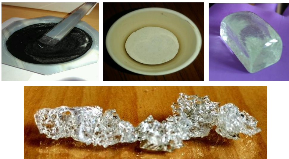
Fig. 4.1 Agro-food waste ashes grounded in agate mortar-pestle, heat-treated ashes, and as-quenched glasses
