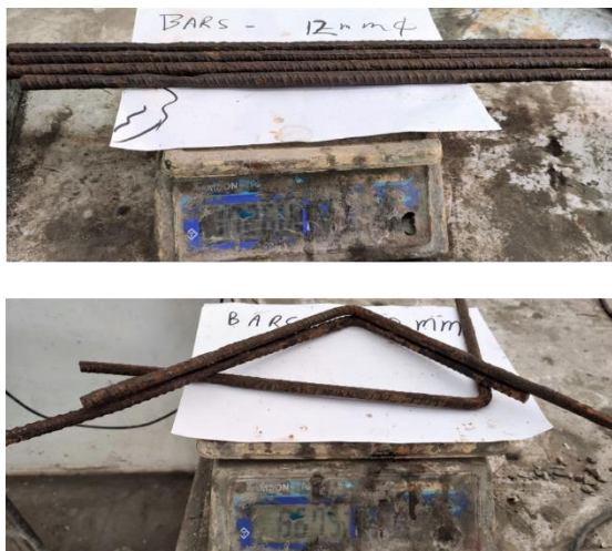
Figure 3. 12 Determining the mass loss for different levels of corroded specimens
