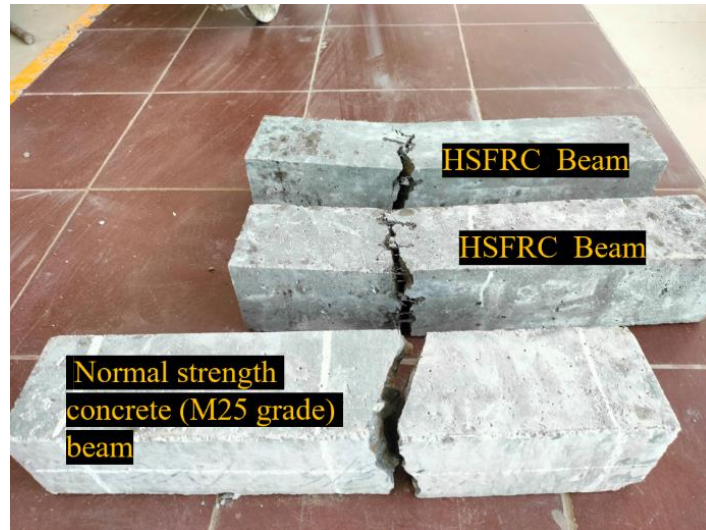
Figure 3. 21 Flexural failure of beam specimens
