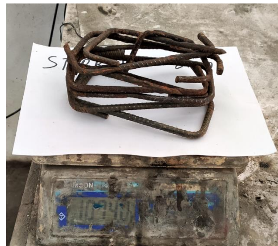
Figure 3. 12 Determining the mass loss for different levels of corroded specimens
