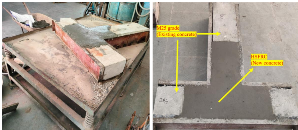
Figure 3. 26 Table vibration provided to the retrofitted specimen
