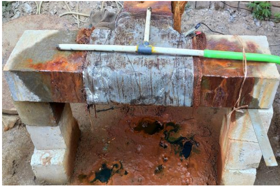
(g) Black liquid oozes out of cracks
