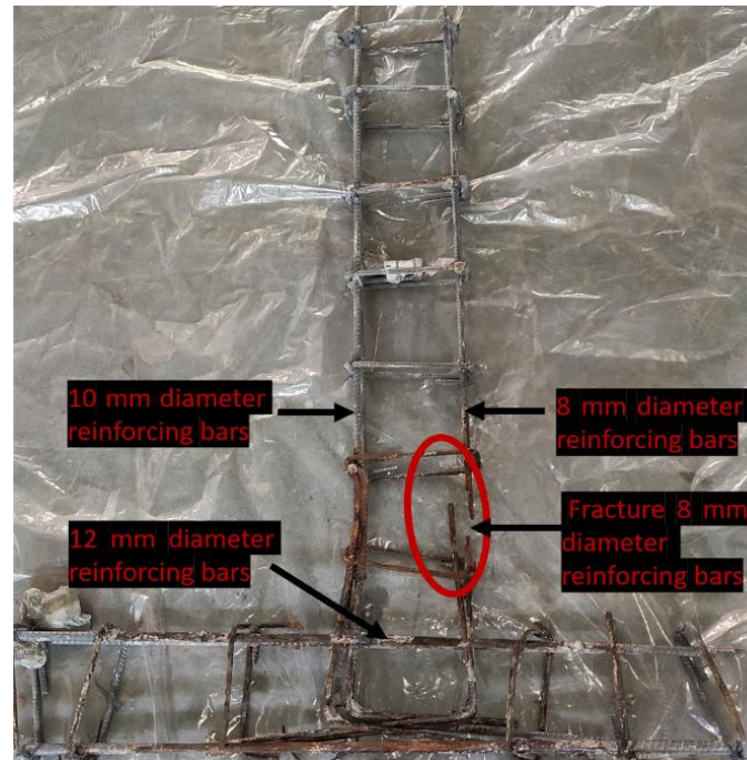
Figure 6. 4 Target corrosion affected length at the reinforcing bars surface (Dangwal and Singh 2023)
