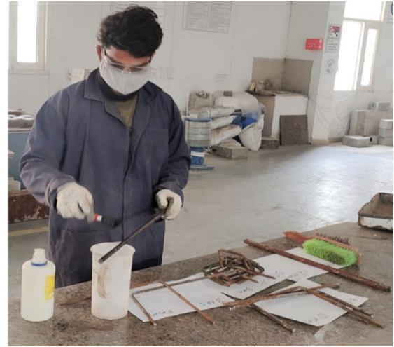
(b) Cleaning and removal of deposited rust
