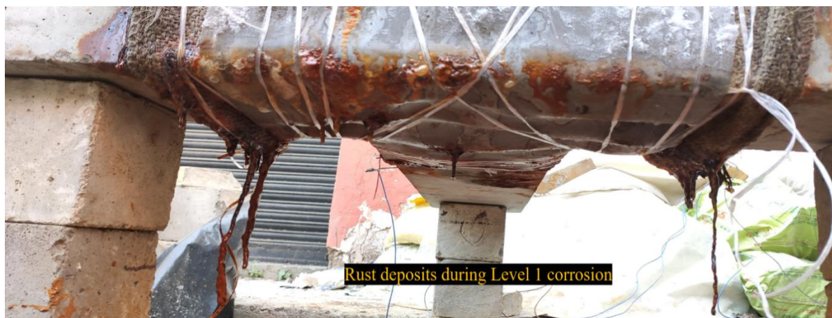
Figure 4. 1 Set-up created for accelerated corrosion and continuous monitoring
