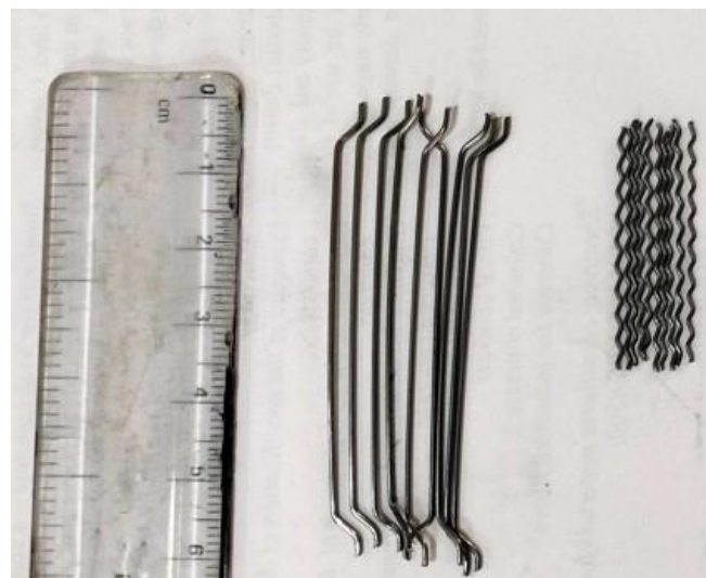
Figure 3. 16 Crimped and hooked-end steel fibers
