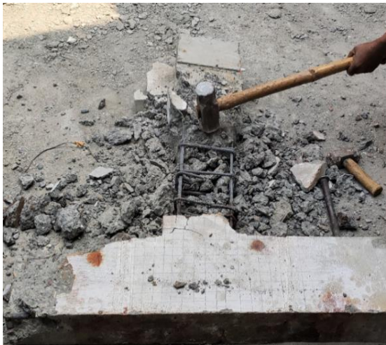
Figure 3. 9 Specimens were distorted after the cyclic loading test for calculating mass loss
