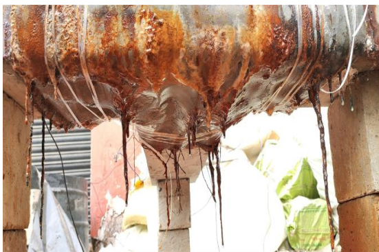
(e) Long suspended peaks of deposited rust
