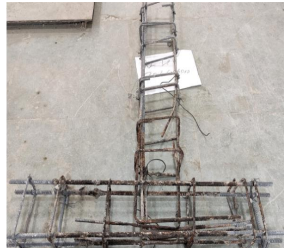
Figure 3. 9 Specimens were distorted after the cyclic loading test for calculating mass loss
