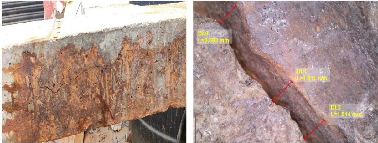
Figure 4. 3 (a) Dense rust deposition and (b) crack width measurement of Level-2 corroded specimen
