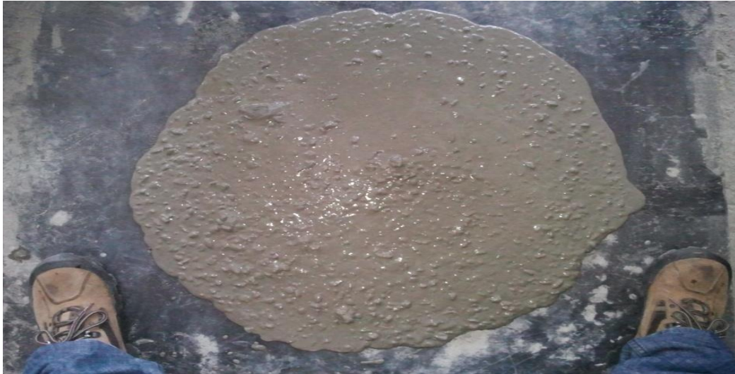
Fig. 4.1: Slump flow test.
