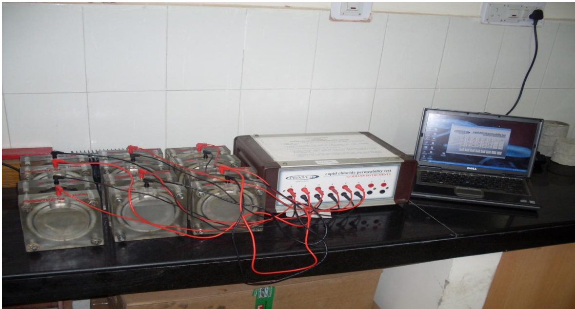
Fig.3.5: Rapid chloride permeability test set up (ASTM C 1202).
