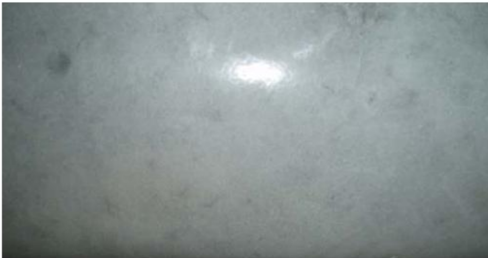
Figure 1.6: Excellent finish of a neat cement SCC (Okamura and Ouchi, 2003a)
