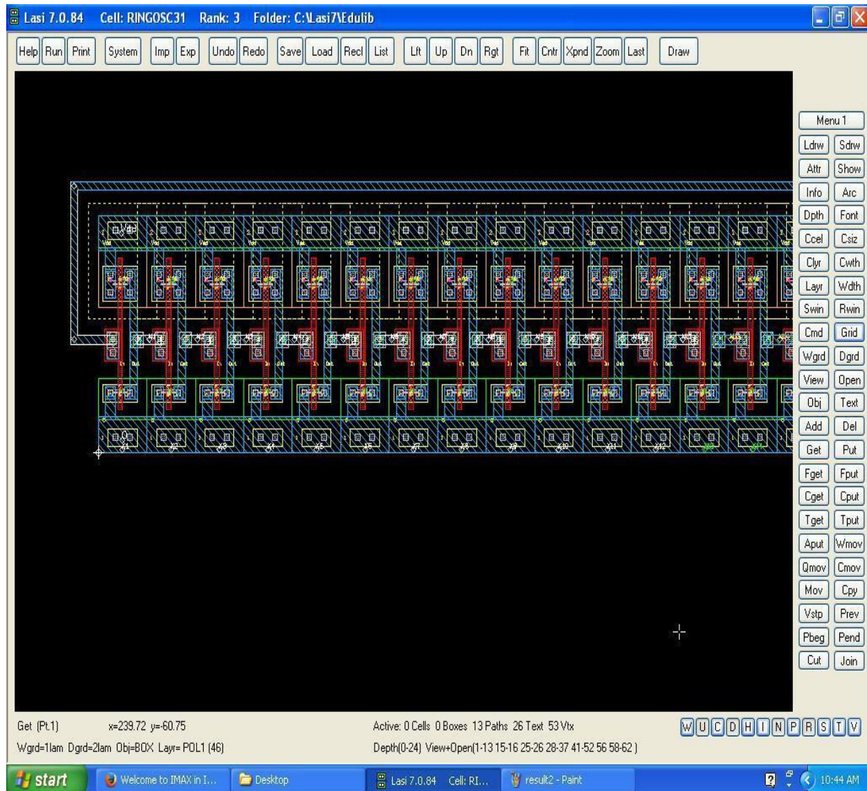
Figure 5.8 Design Layout of VLSI Circuit (Ring Oscillator) Using Ozone Oxidized FinFETs.
