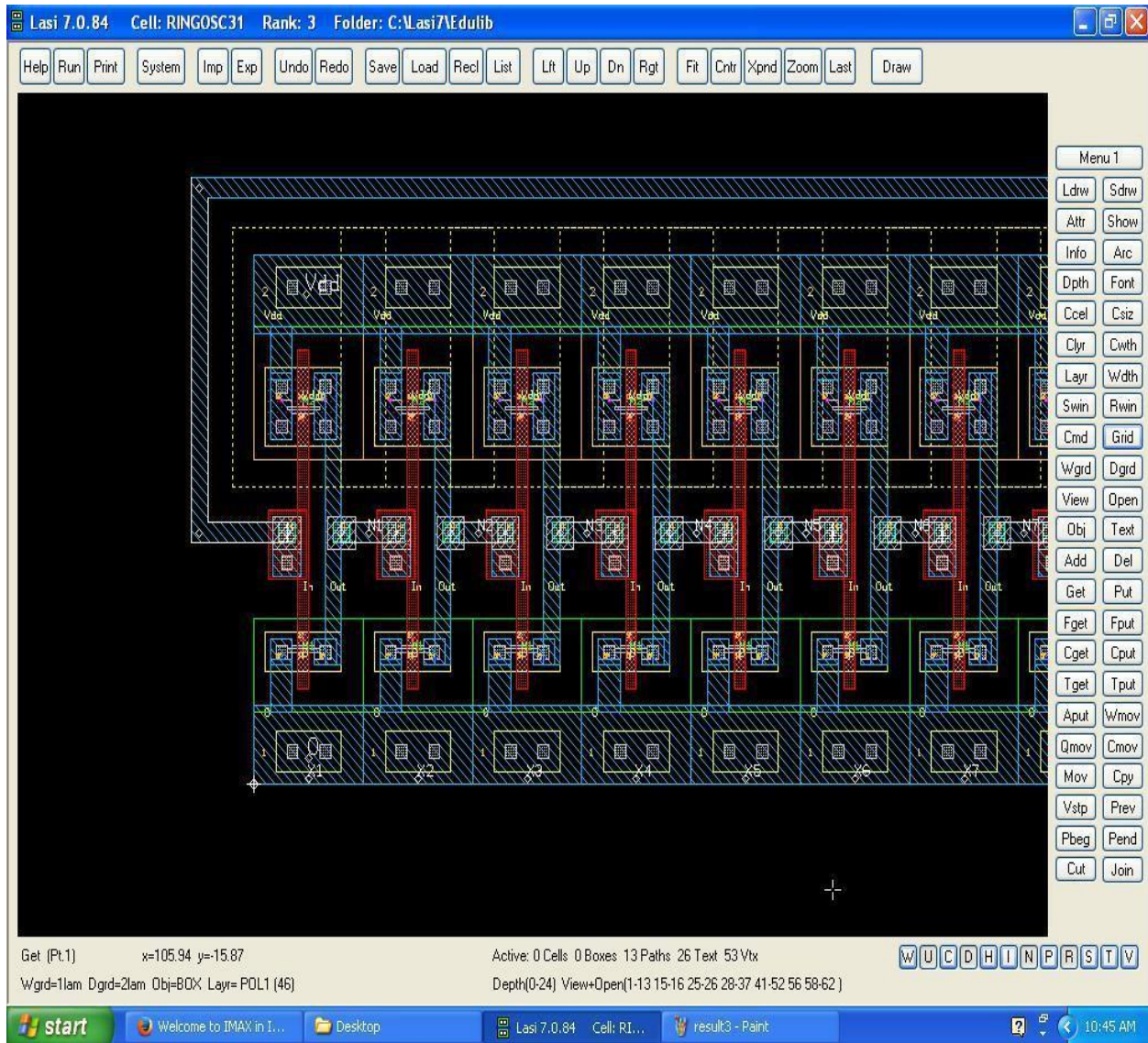
Figure 5.9 Zoom in figure of the design layout of the 31-stage ring oscillator using ozone oxidized FinFETs.
