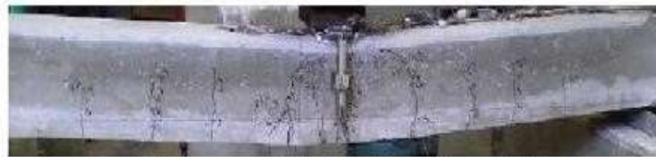
3) Flexural failure of specimen C2
