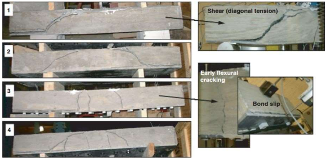
Fig.2.21 Failure Modes Specimens 1 to 4 ( Honickman et al. (2009) )
