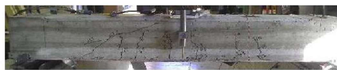
a) Shear failure of specimen 1
