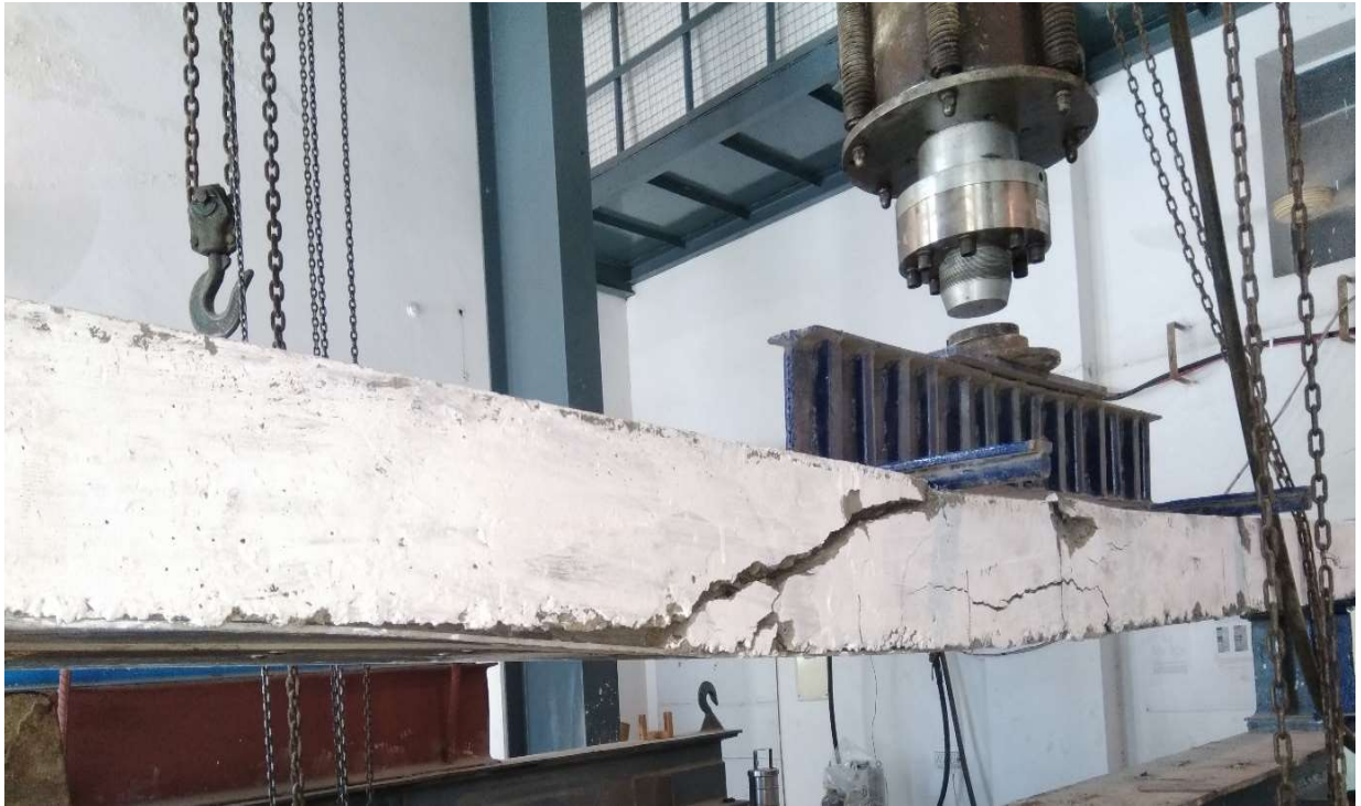
Fig 4.19 Crack pattern of Specimen SLB 0 after final stage
