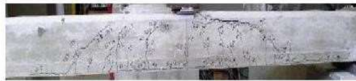
1) Hybrid failure mode of specimen 4
