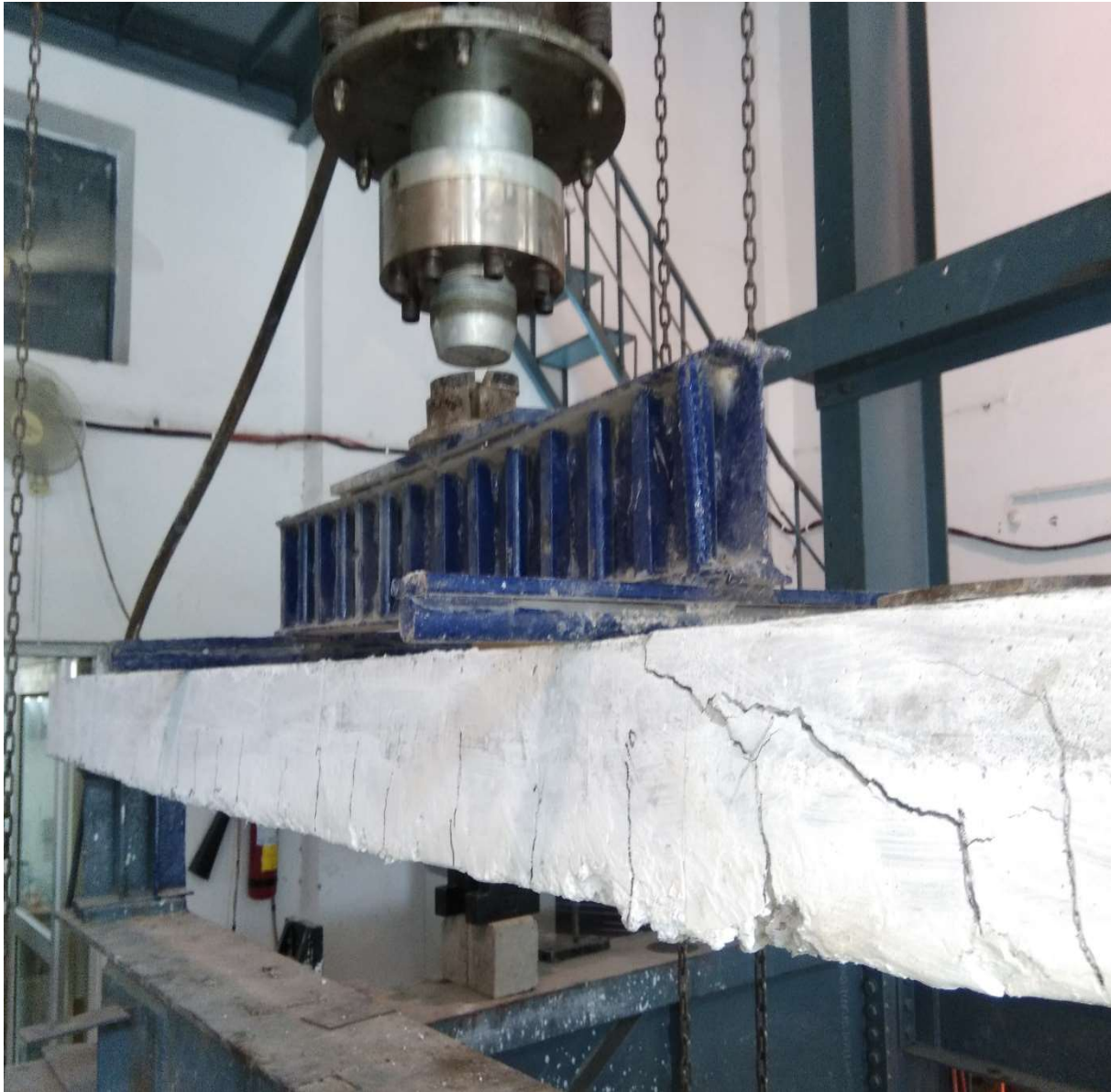
Fig 4.15 Shear cracks on specimen SLA
