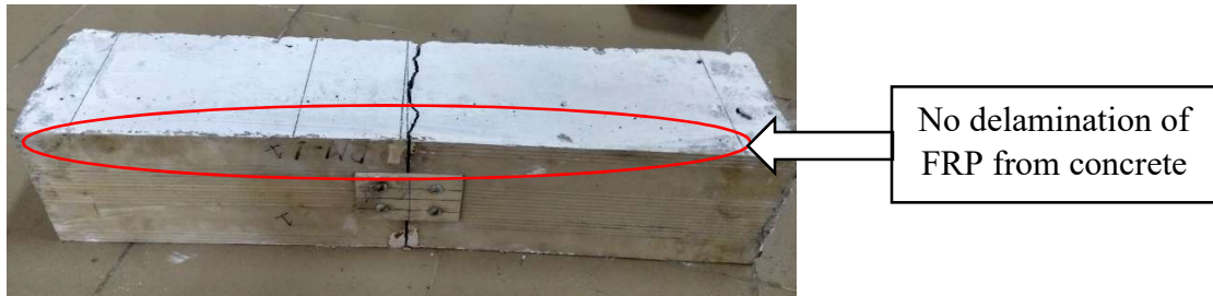
Fig 4.13 Flexure cracks on specimen BTB 0
