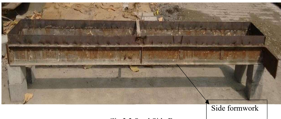
Fig.3.3 Steel Side Form
