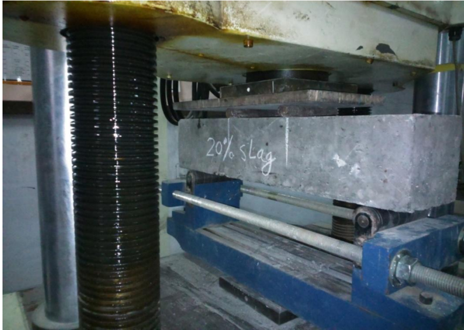
Fig 4.10 Test setup for flexural strength
