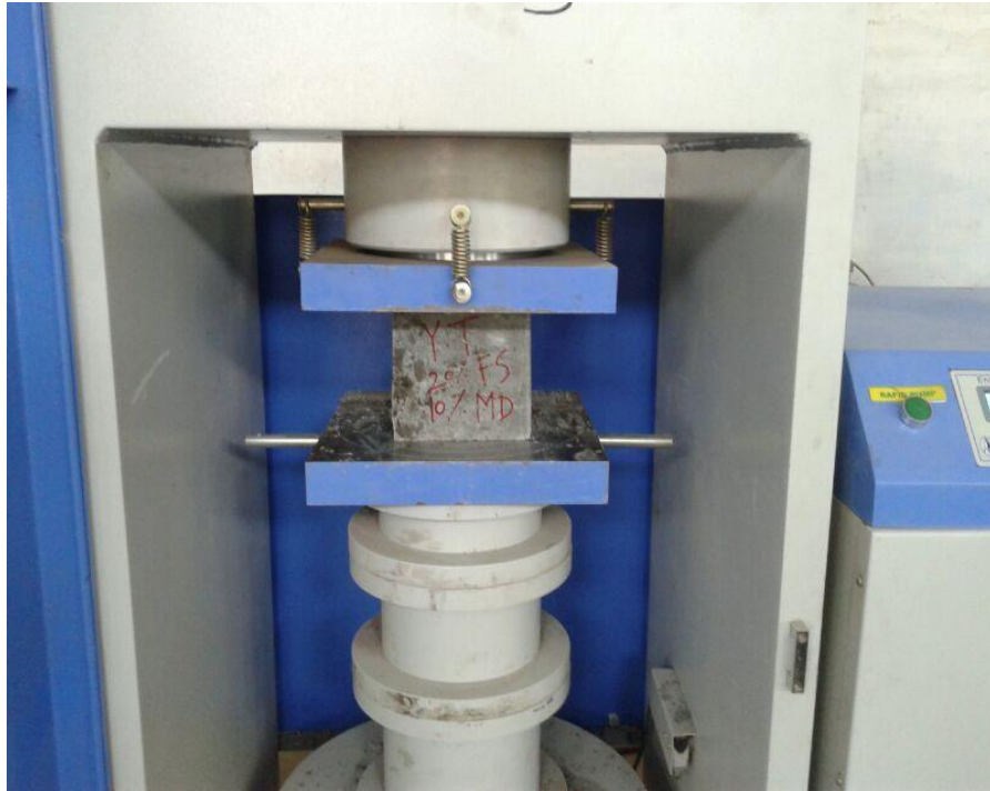
Fig 4.1 Compressive strength test setup
