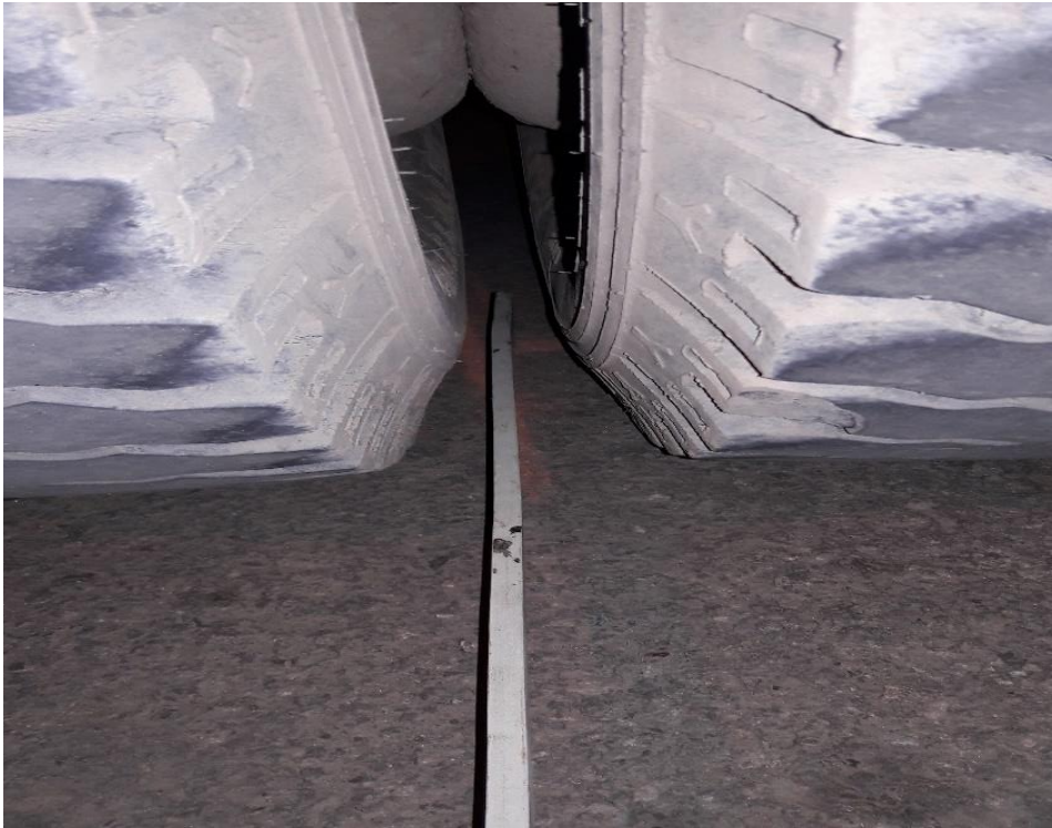
Fig. 3.8: Placement of Beam Probe in between Rear Tires of Truck
