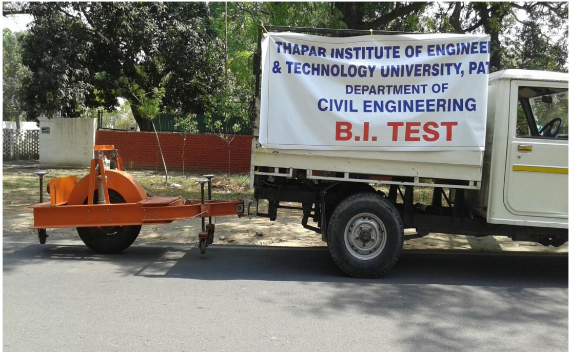
Fig. 3.27: Bump Integrator Test (Roughness Test) in Progress on Section UR03 (Chopra, T, Parida, M, Kwatra, N, Mandhani, J. (2017))
