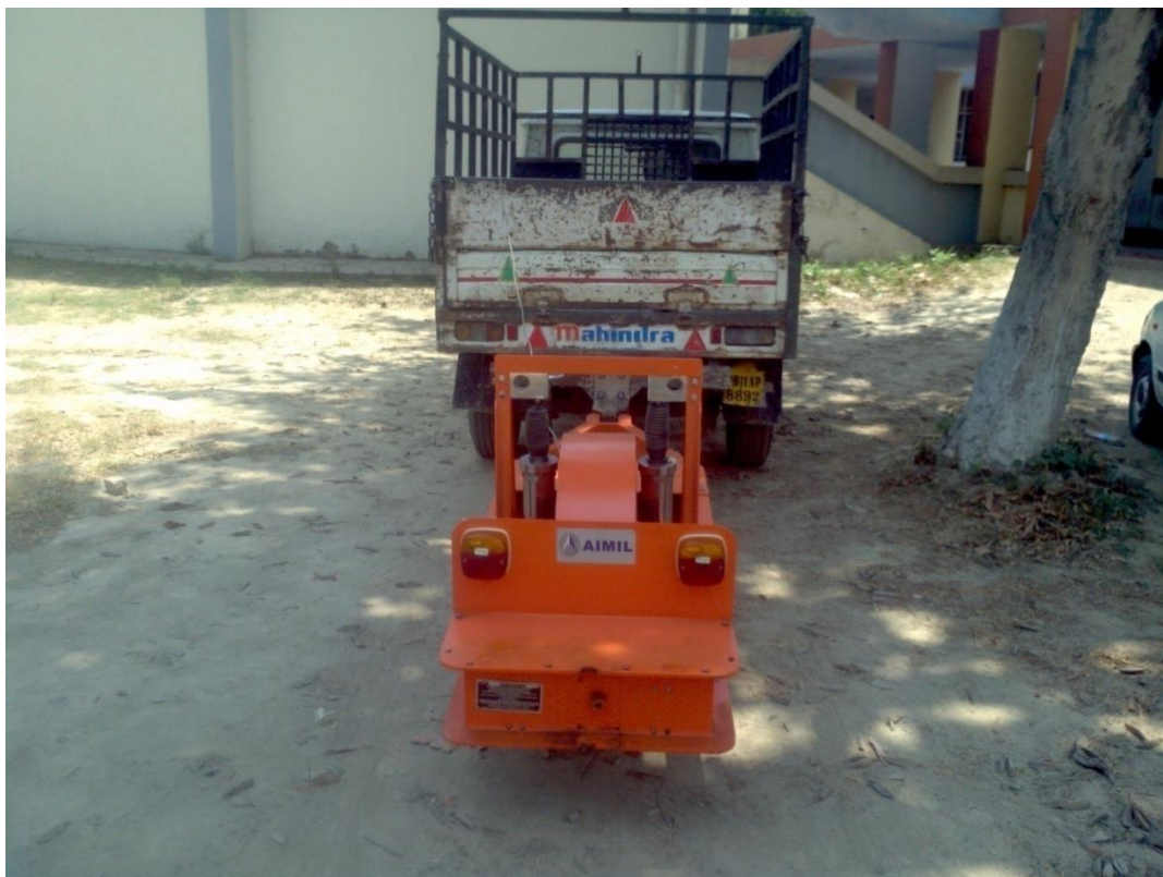
Fig. 3.26: Bump Integrator (Roughometer) Towed with Pick-up
