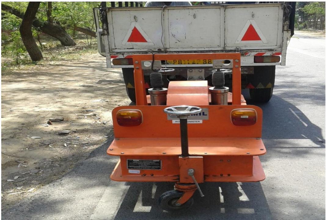
Fig. 3.28: Bump Integrator Test in Progress on Section UR03
