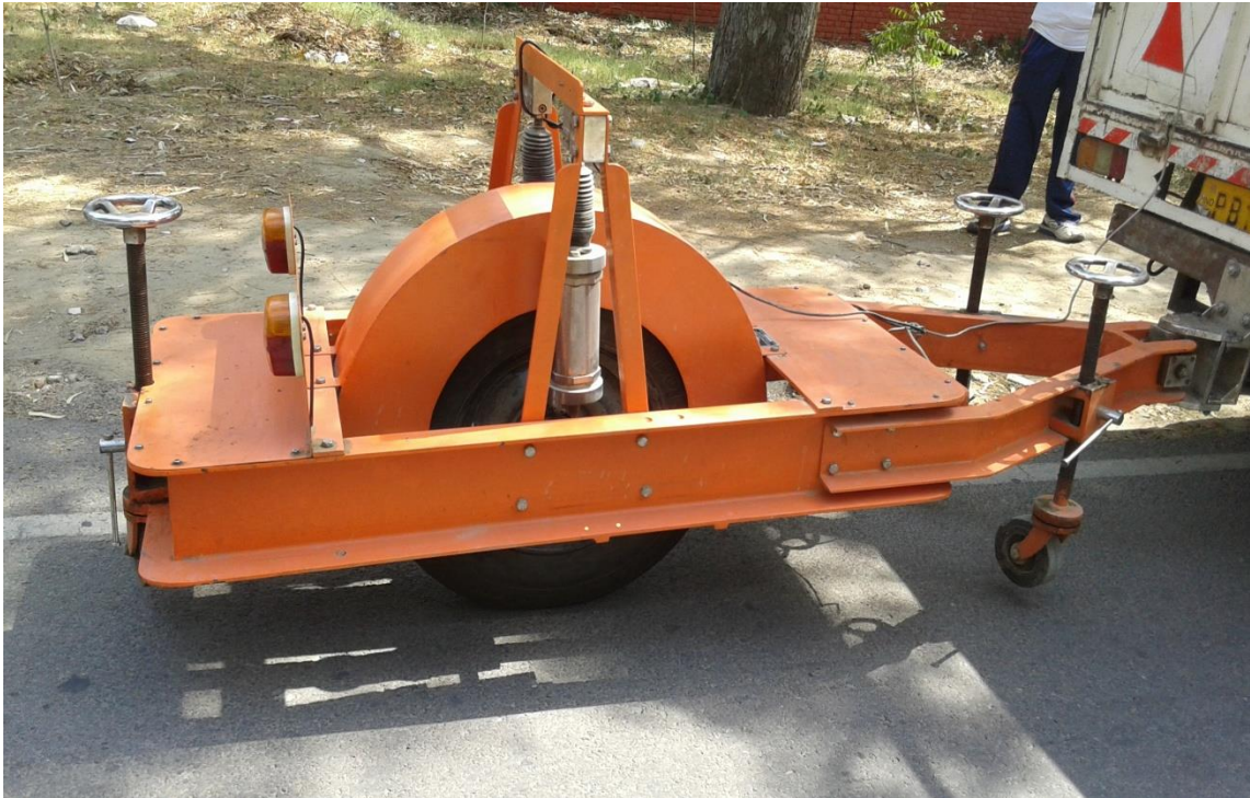
Fig. 3.29: Bump Integrator Test in Progress on Section UR04
