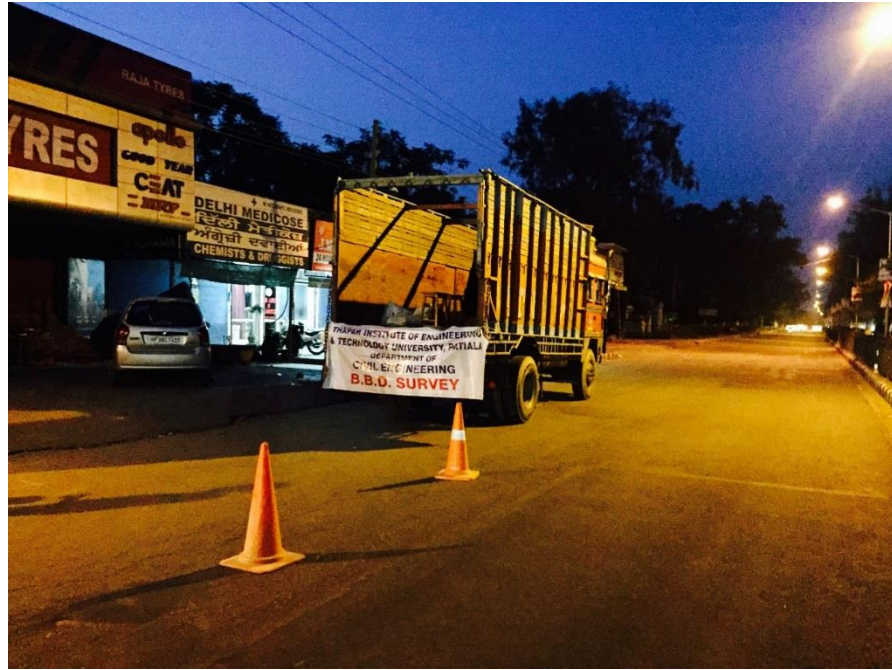
Fig. 3.10: BBD Test as per IRC 81 guidelines
