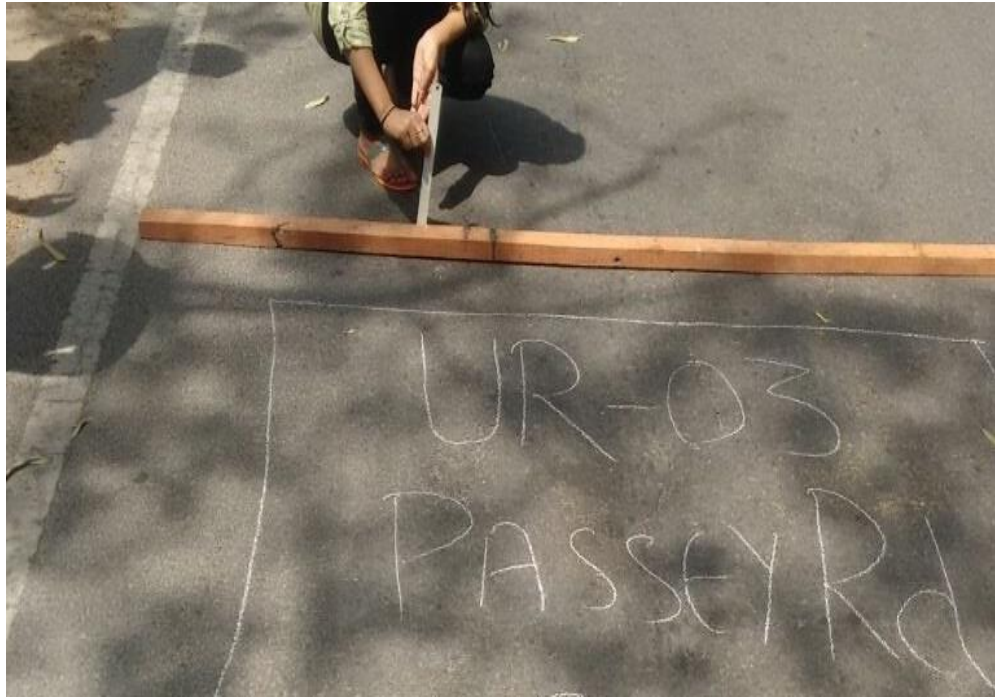
Fig. 3.24: Rut Depth Measurement on Section UR03
