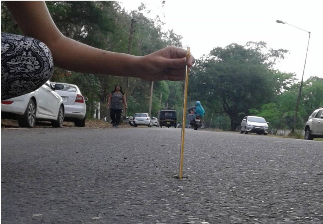
Fig. 3.11: Determination of Actual Pavement Temperature on Road Section UR03
