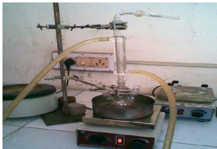
Fig 2.3 Experimental setup for co-precipitation method
