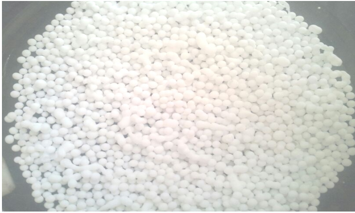
Figure 4.3: TiO 2 entrapped Alginate balls.
