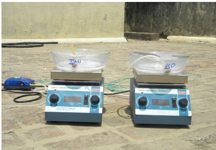
Figure4.2: Shallow pond slurry type reactor
