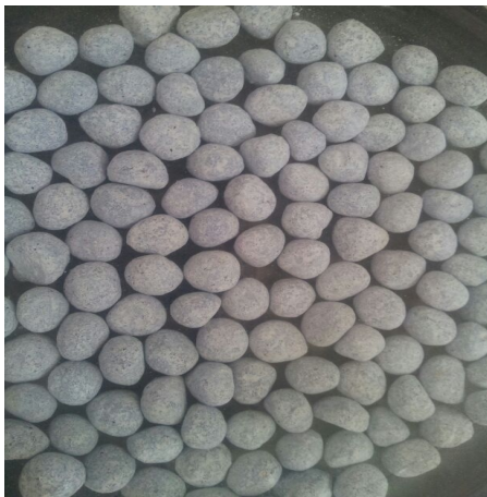
Figure 4.4: TiO 2 immobilized cement beads.
