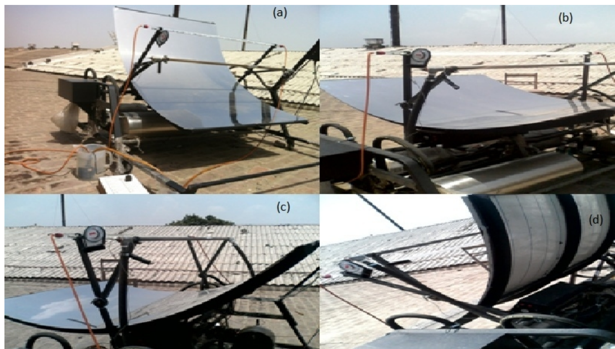
Figure 5.12: Representation of Solar Parabolic Collector at the angle of inclination of (a) - 40^\circ (b) 0^\circ (c) 20^\circ (d) 40^\circ respectively.
