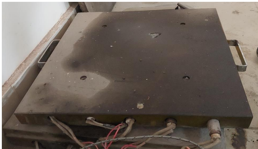
Figure 3.8 Square 400 mm heating plate used for the elevated temperature set-up
