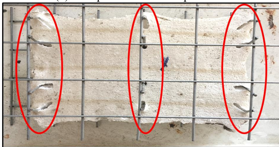
(b) EPS panel skeleton exposed to 100 0 C
