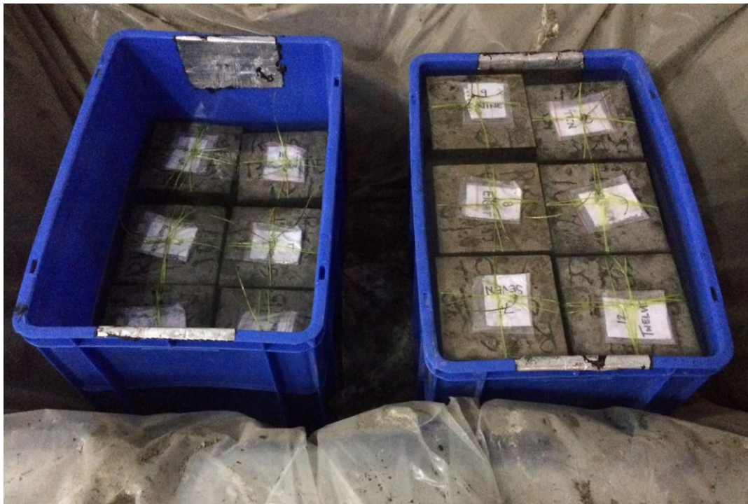
Fig.3.18 Sulphate resistance test
