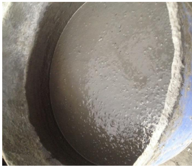
Fig.3.8 Preparation of SCC
