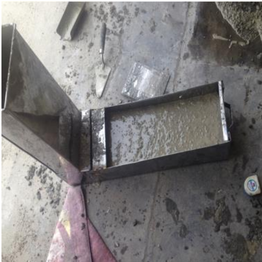
Fig.3.12 L-box test for SCC
