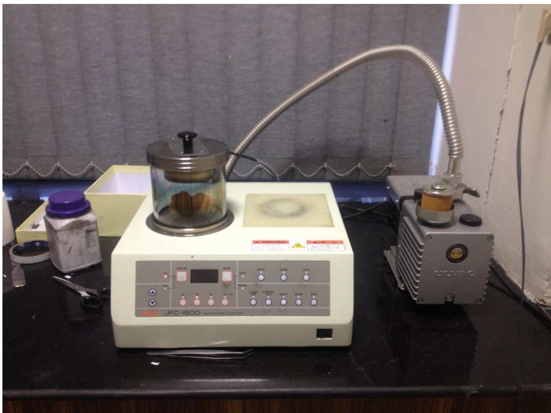
Fig.3.20 Coating of sample before SEM
