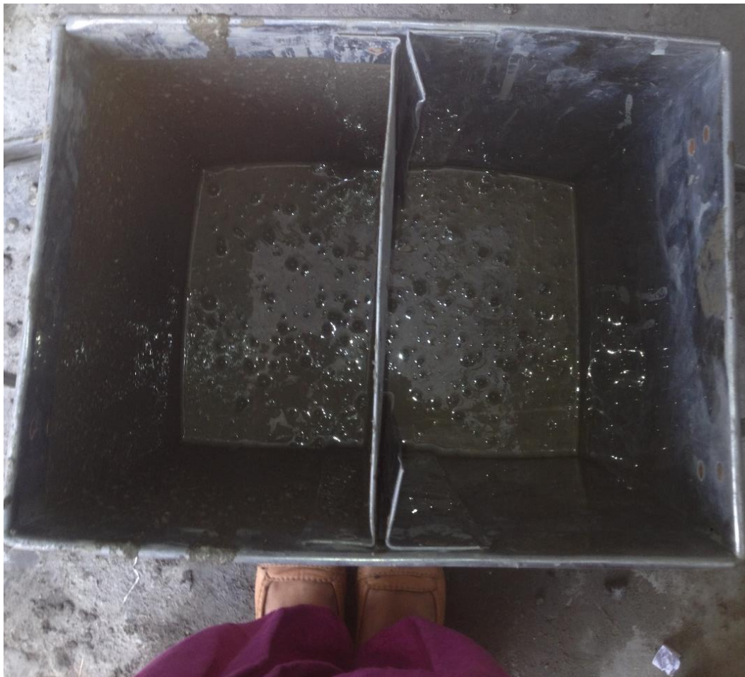
Fig.3.13 U-box test SCC
