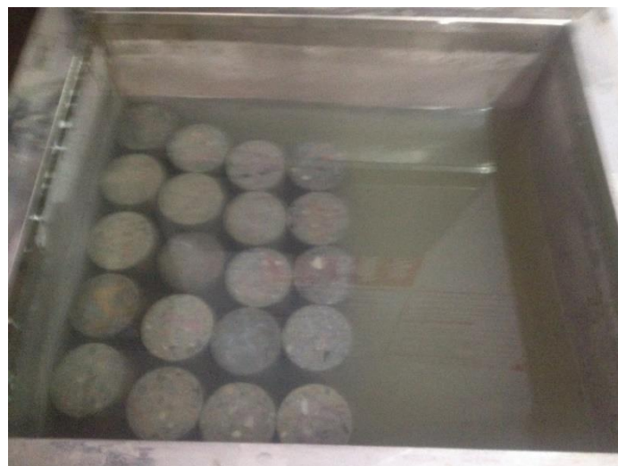
Fig.3.16 Water absorption test
