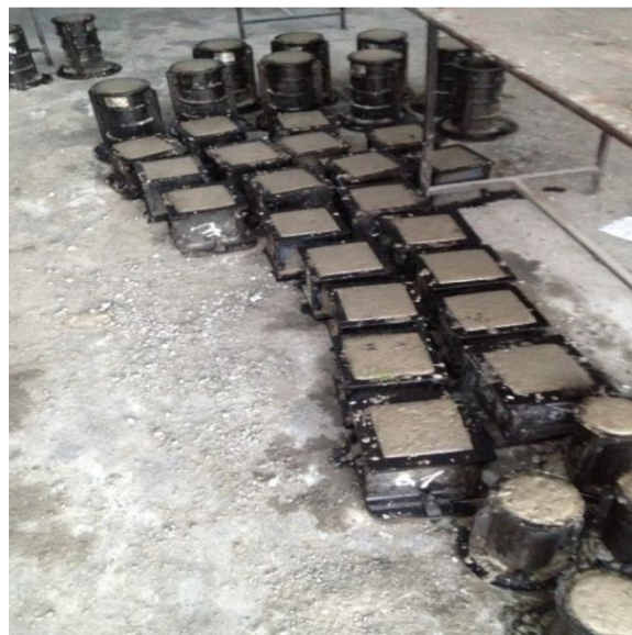
Fig.3.9 Casting of specimens
