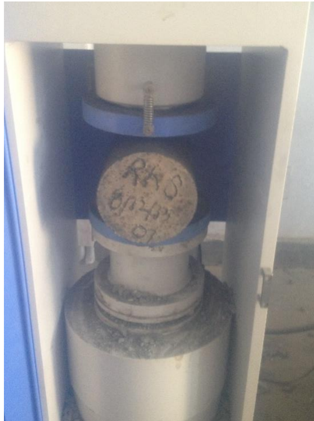
Fig.3.15 Splitting tensile strength test
