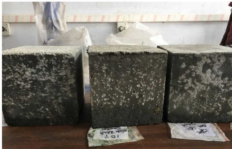
Fig. 4.45 SCC specimens after 365 days of sulphate attack
