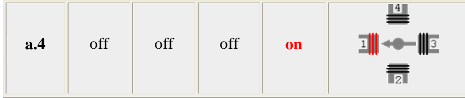
Figure-5.12 Single-Coil Excitation
