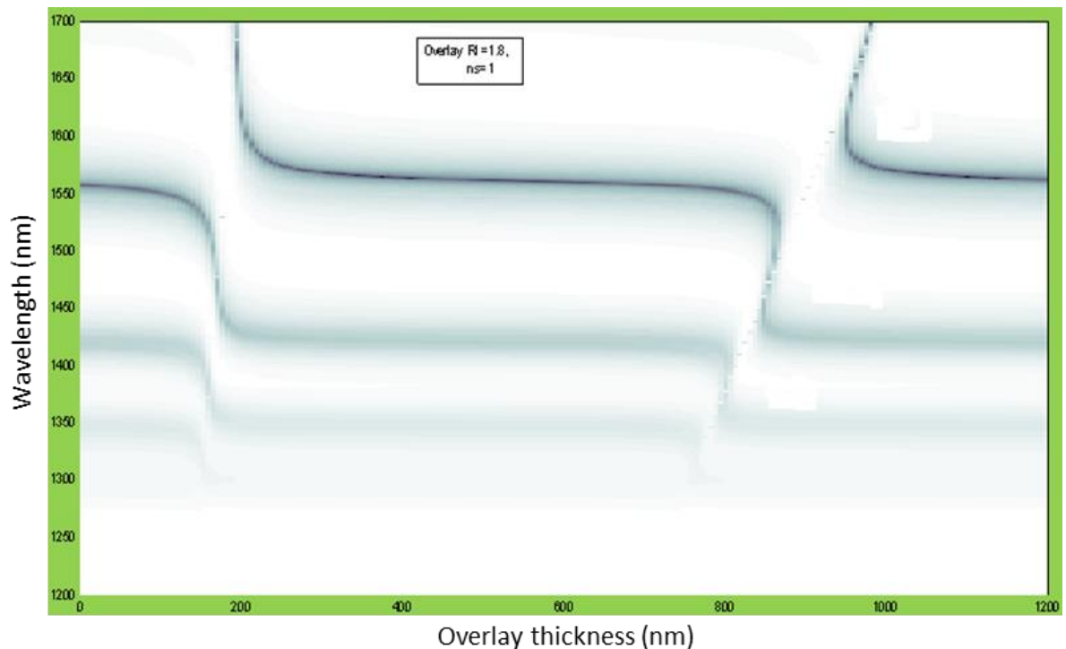
Figure 5.3 Growth of various cladding mode resonances as a function of overlay thickness (1.8) and refractive index n_s=1
