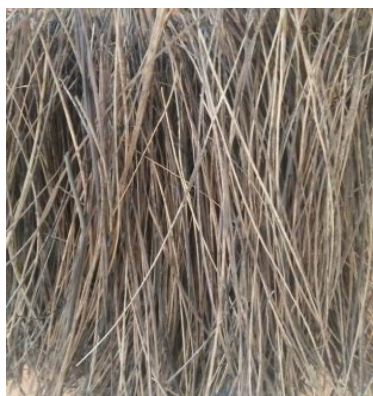
Figure 3.2 Fibers after 1% stearic acid treatment
