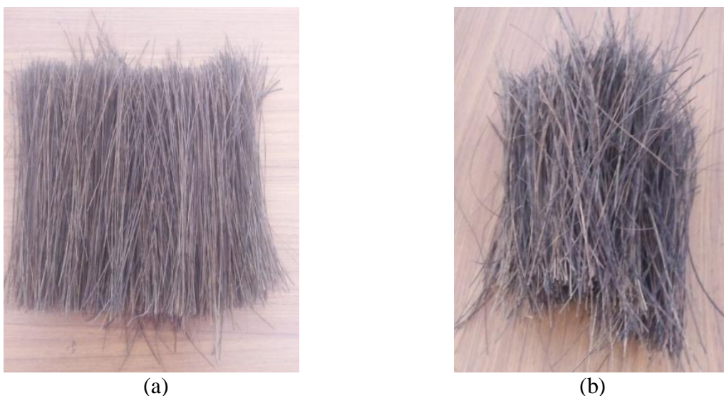
Figure 3.1 (a) Fibres before alkali treatment and (b) Fibres after alkali treatment
