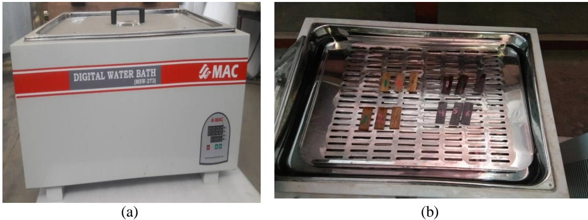
Figure 4.6 (a) Water bath chamber and (b) Specimens in water bath chamber
