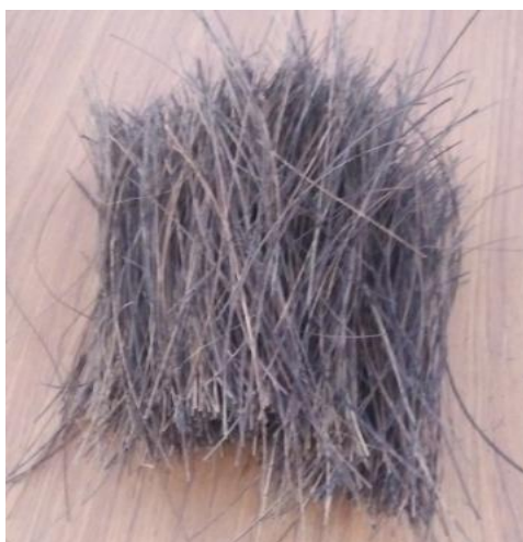
Figure 3.3 Fibres after 4% stearic acid treatment
