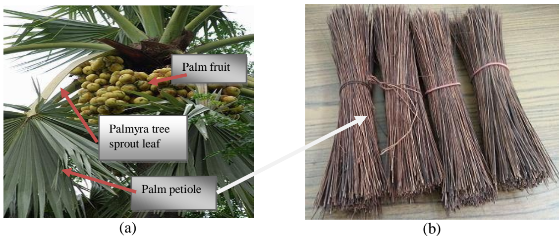
Figure 1.5 (a) Different resources of fibres in Palmyra Palm tree and (b) Extracted ‘Palmyra Palm Petiole’ fibre (Borrassus Flabelliformis) [10]
