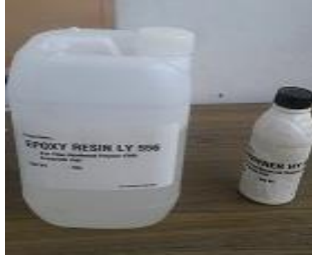
Figure 4.1 Epoxy Resin LY 556 and Hardener HY 951
