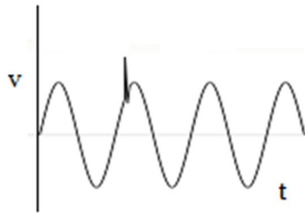
Figure-2.4: Voltage Spike
