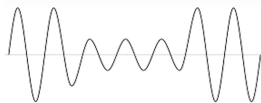
Figure-2.1: Voltage Sag
