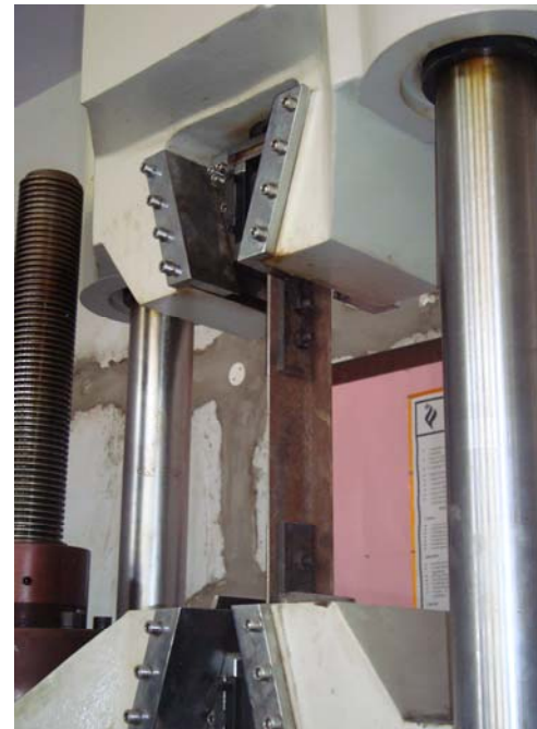
Fig. 3.4: Specimen grip assembly in UTM
