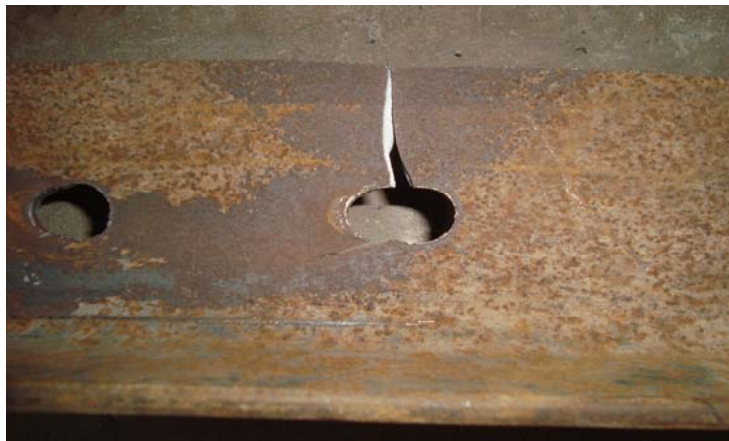
Fig. 3.19: Partial net section rupture, with small eccentricity (specimen 6)
