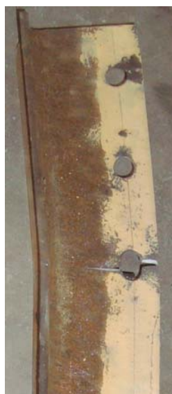
Fig. 3.20: Partial net section rupture, with large eccentricity (specimen 4)
