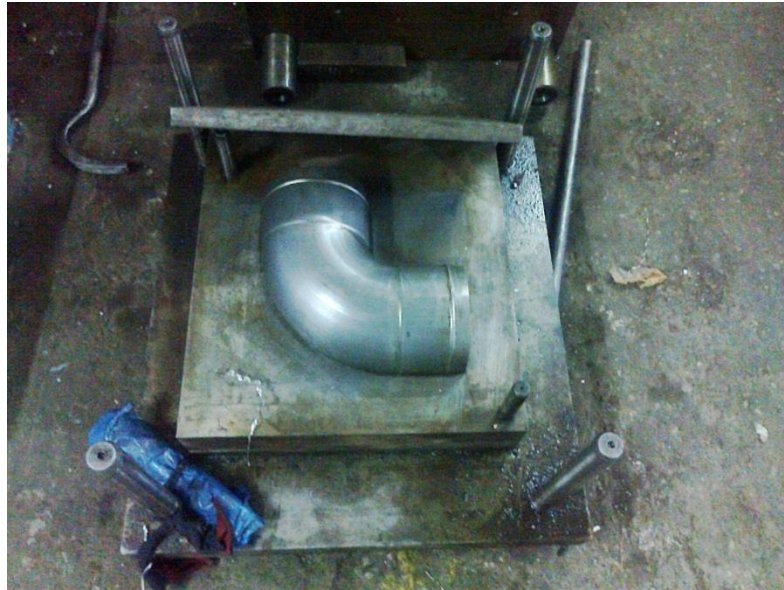
Figure 5.2 Tool used for Deep Draw
