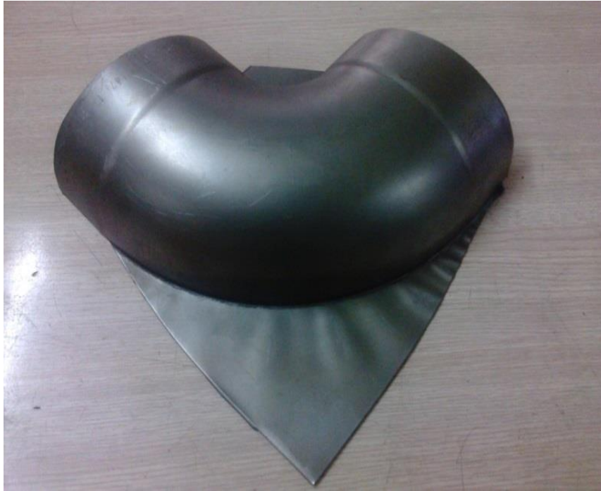
Figure 3.1 Wrinkling in Component
