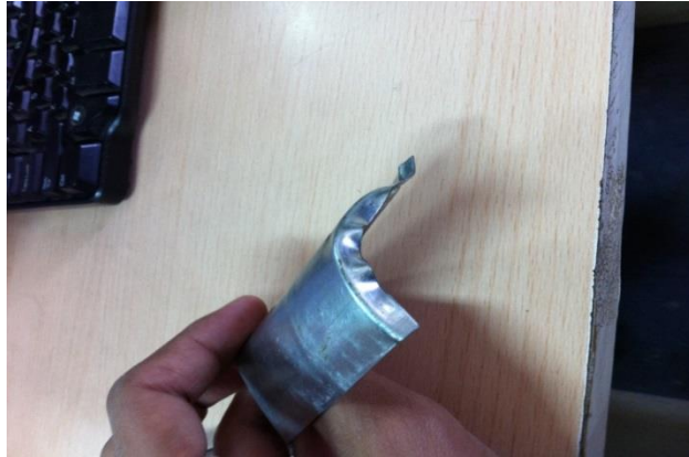
Figure 2.2 wrinkling on the part
