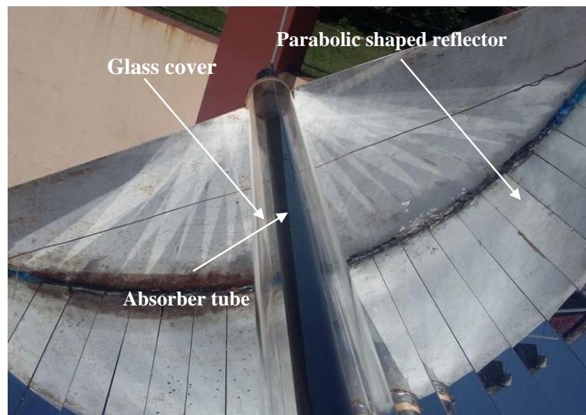
Figure 4.2 Parabolic reflector and absorber tube along with glass cover
