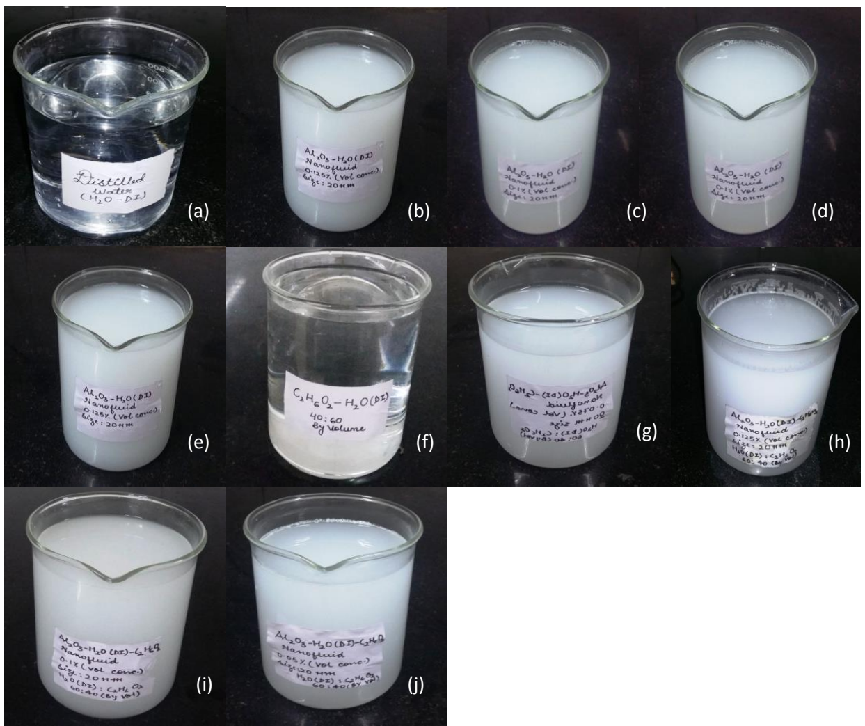
Figure 4.12 various prepared working fluid: (a) Distilled water, (b) 0.05% vol. conc. Al 2 O 3 -H 2 O (DI), (c) 0.075% vol. conc. Al 2 O 3 -H 2 O (DI), (d) 0.1% vol. conc. Al 2 O 3 -H 2 O (DI), (e) ) 0.125% vol. conc. Al 2 O 3 -H 2 O, (f) H 2 O-C 2 H 6 O 2 (60:40 by volume), (g) 0.05% vol. conc. Al 2 O 3 -H 2 O- C 2 H 6 O 2 (60:40 by volume), (h) 0.075% vol. conc. Al 2 O 3 -H 2 O- C 2 H 6 O 2 (60:40 by volume), (i) ) 0.1% vol. conc. Al 2 O 3 -H 2 O- C 2 H 6 O 2 (60:40 by volume) and (j) 0.125% vol. conc. Al 2 O 3 -H 2 O- C 2 H 6 O 2 (60:40 by volume)
