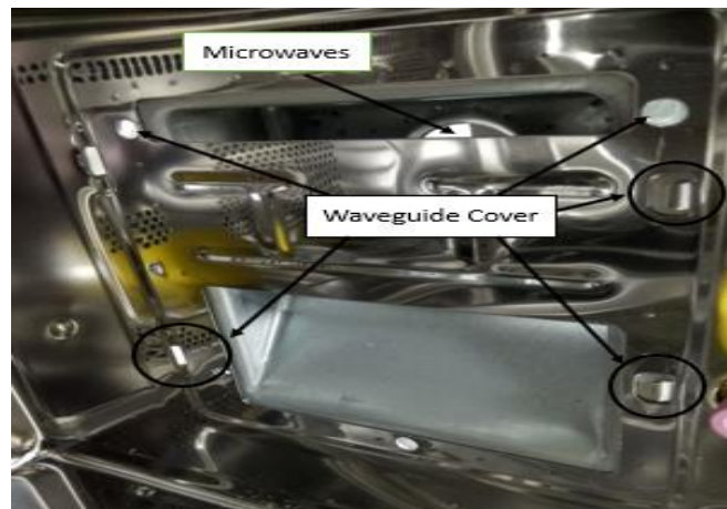
Figure 3.7: Waveguide in The Microwave Oven
