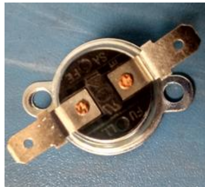
Figure 3.10: Thermostat in Microwave Oven
