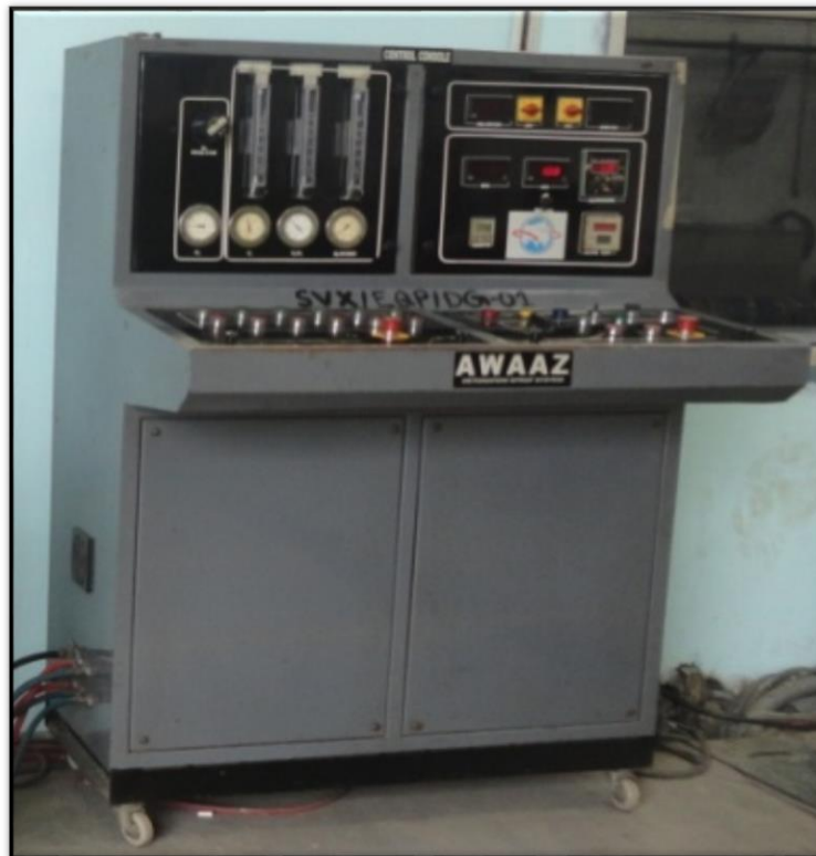
Figure 3.2: Control panel of Detonation gun spray process (courtesy SVX Company Greater Noida UP)
