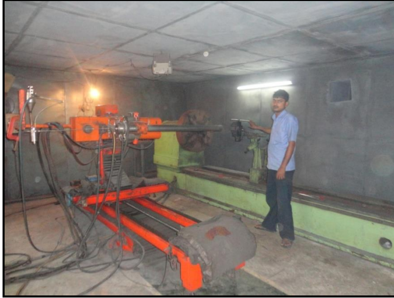
Fig 3.1: Image of detonation gun apparatus.(courtesy SVX company Greater Noida)
