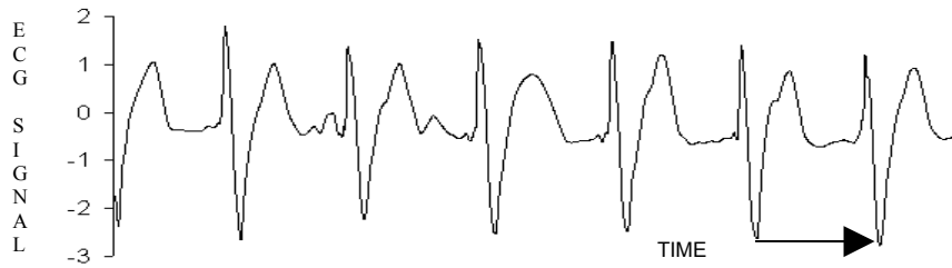
Figure 6.3: Reconstructed ECG for patient 107, lead MLII, CR =24
