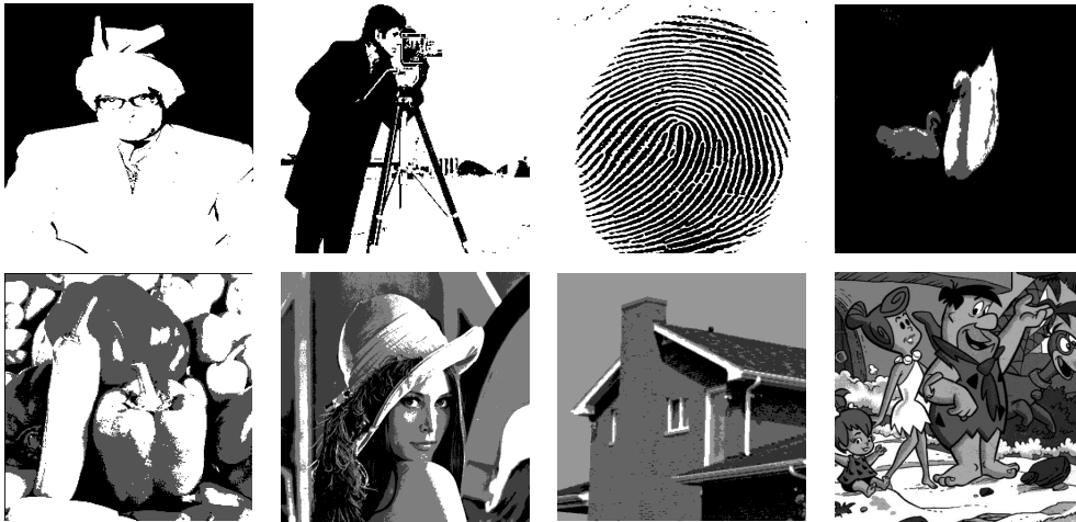
Figure 5.10: Segmented images of the experimental image data set using FODPSO technique: (a) Man, (b) Cameraman, (c) Fingerprint, (d) Two Swans, (e) Peppers, (f) Lena, (g) House, and (h) Flinstones.
