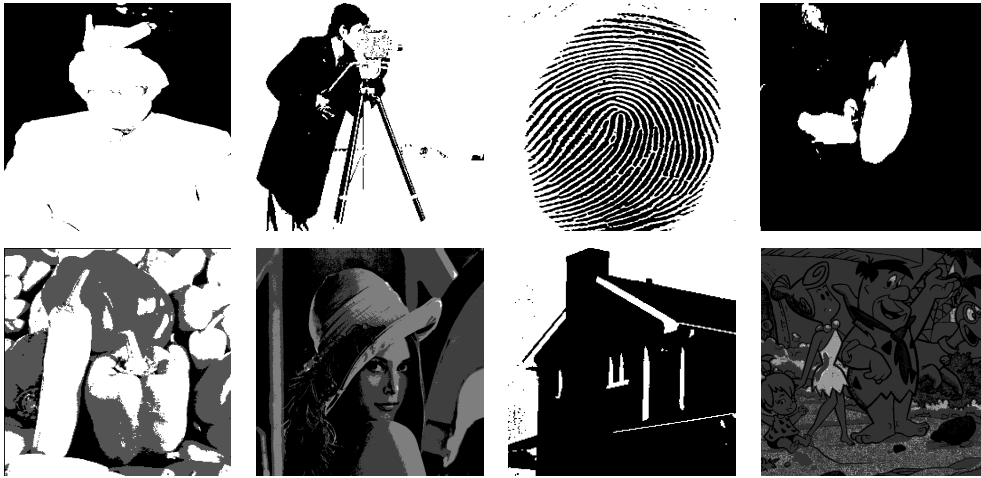
Figure 4.5: Segmented images with respect to optimal thresholds obtained by proposed technique using histogram of the images: (a) Man, (b) Cameraman, (c) Fingerprint, (d) Two Swans, (e) Peppers, (f) Lena, (g) House, and (h) Flintstones.
