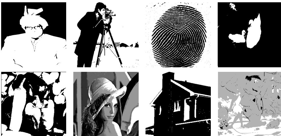
Figure 4.6: Segmented images with respect to optimal thresholds obtained by proposed technique using energy curve of the images: (a) Man, (b) Cameraman, (c) Fingerprint, (d) Two Swans, (e) Peppers, (f) Lena, (g) House, and (h) Flintstones.
