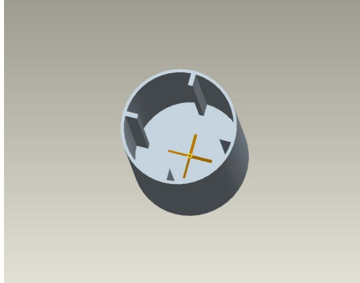
Figure 5.6 Assembly of propeller and cylindrical tank
