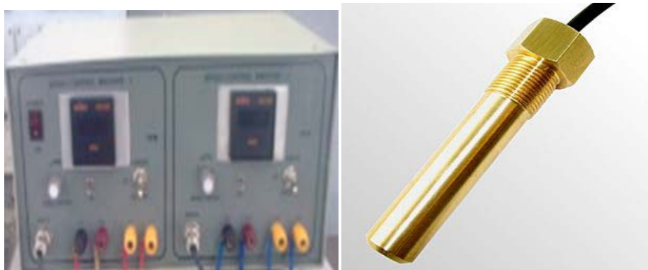
Figure 5.3 Speed control unit and magnetic rpm sensor
