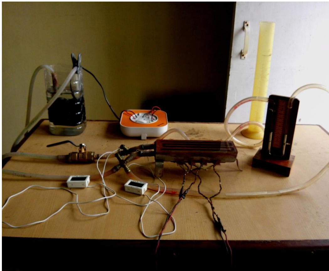
Figure 4.1 Experimental setup for Mini-channel based Heat Sink (MCHS) cooling system
