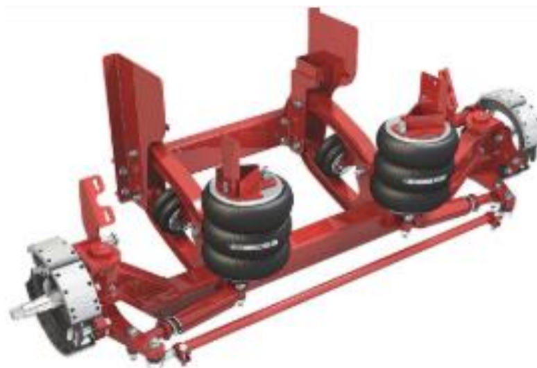
Figure 5.30: 3D CAD model of lift axle suspension [30]
